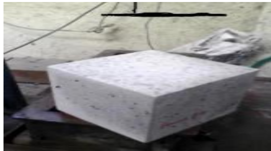
FIGURE 1.1 Light weight mortar cube
