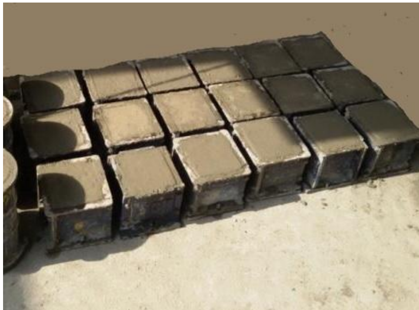
Figure 5.2: Specimen for compressive and flexural test.
