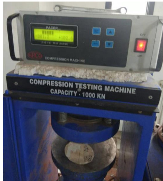
Figure 9: Split Tensile Test of Cylinder
