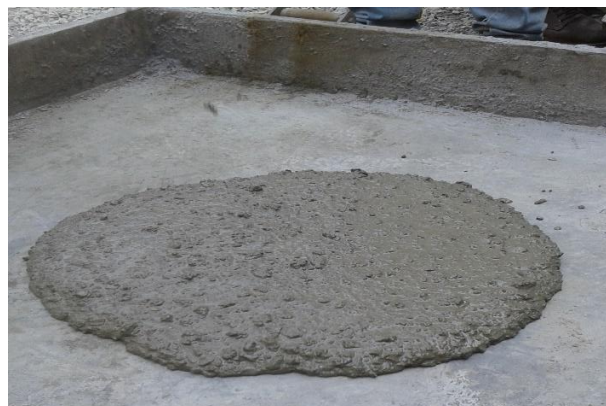
Figure 6: Slump Test of Concrete
