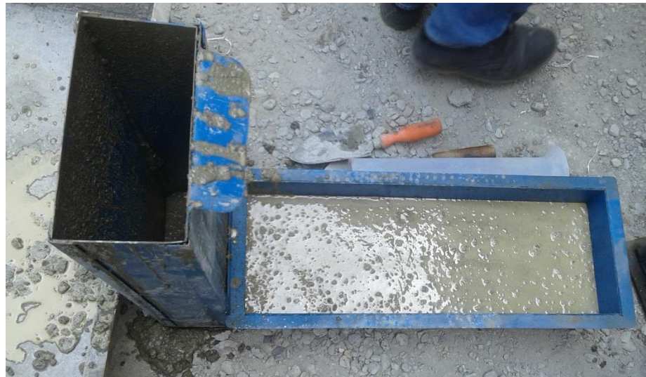
Figure 7: L-Box Test of Concrete
