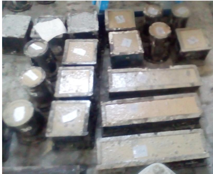
Figure 11: SCC Mix in mould
