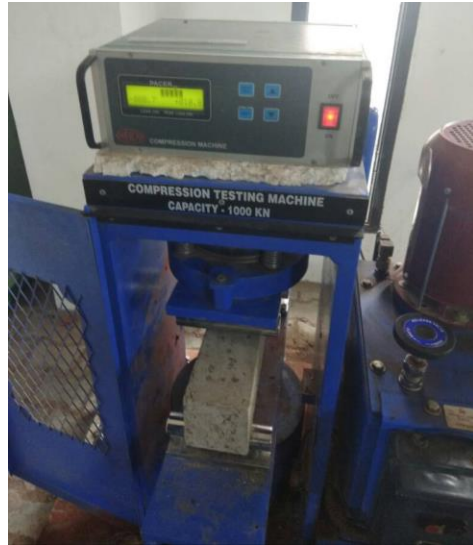
Figure 10: Flexural Test of Beam
