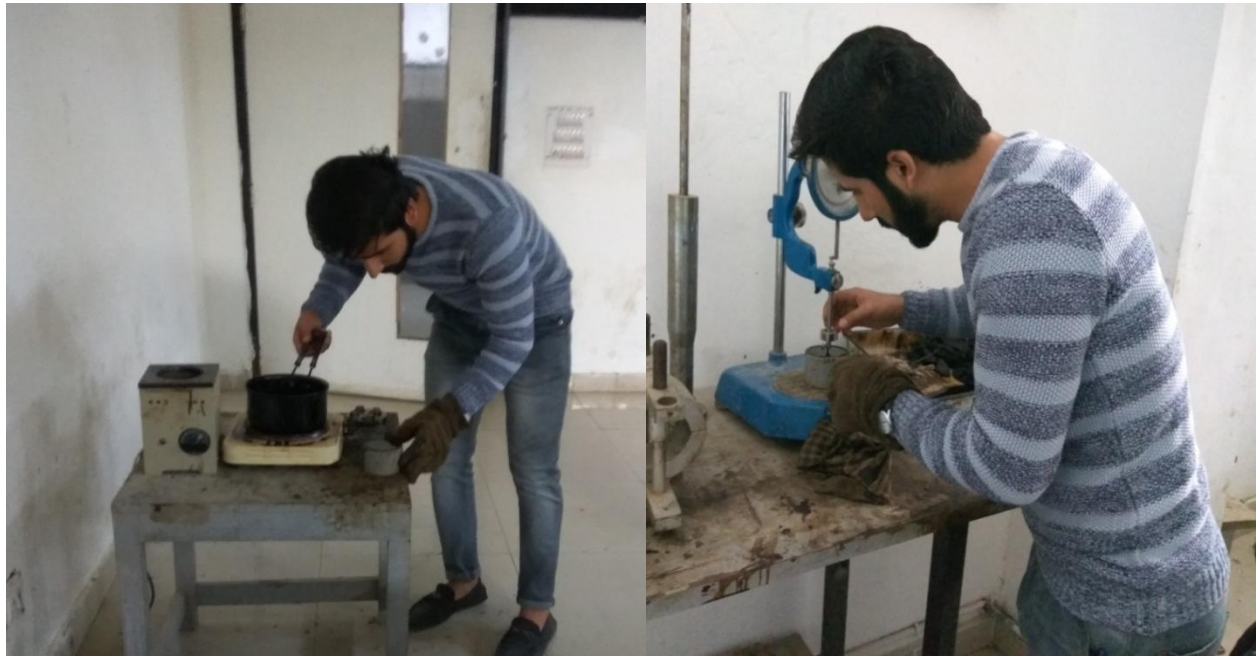
Figure 4.6: various steps involved in penetration test
