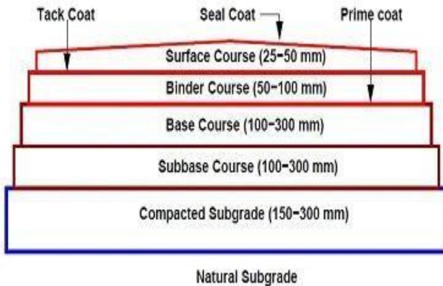
Figure 1.5 showing different layers of bitumen
