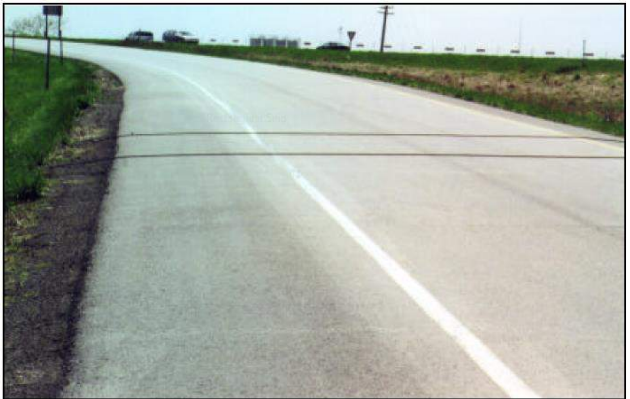
Fig.3.81: pneumatic road tubes (source: google image)
