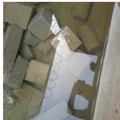
Fig 7.5 Curing of cubes and cylinders
