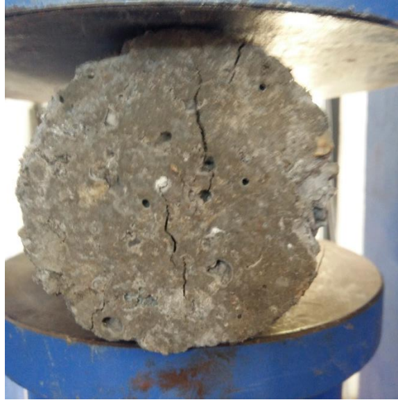
Fig 7.14 Split tensile strength of plastic setup
