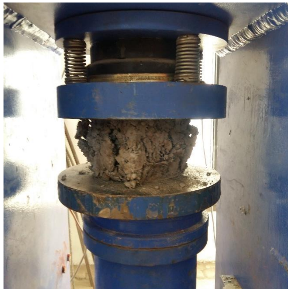
Fig 7.12 compressive strength of plastic test setup
