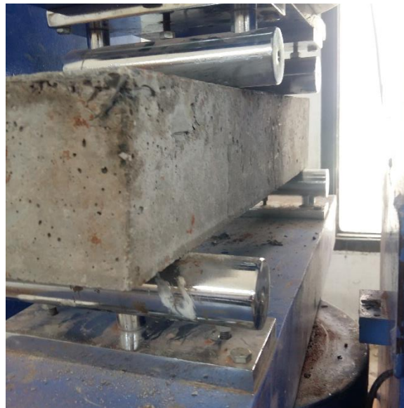
Fig 7.10 Flexural Strength Setup
