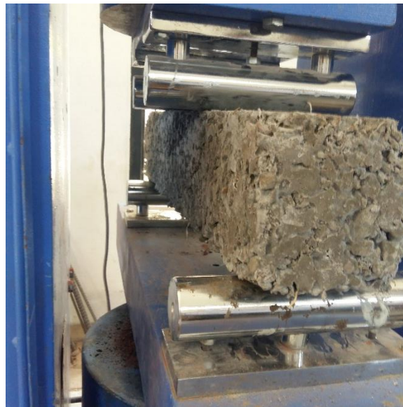
Fig 7.16 Flexural strength test of plastic aggregates setup
