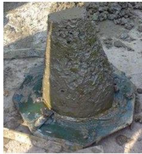
Figure 2 Slump Test for trial mix
