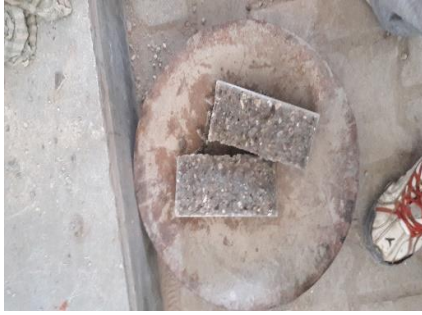
Figure 4 Failure of control specimen WA
