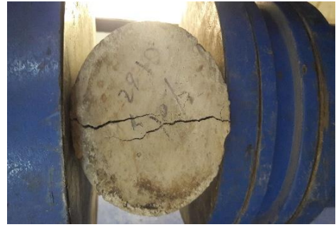
Figure 5 Failure of Specimen along WA
