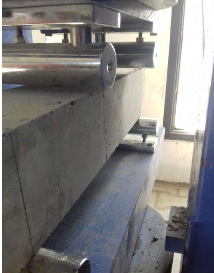
Fig 20: Flexural Strength testing
