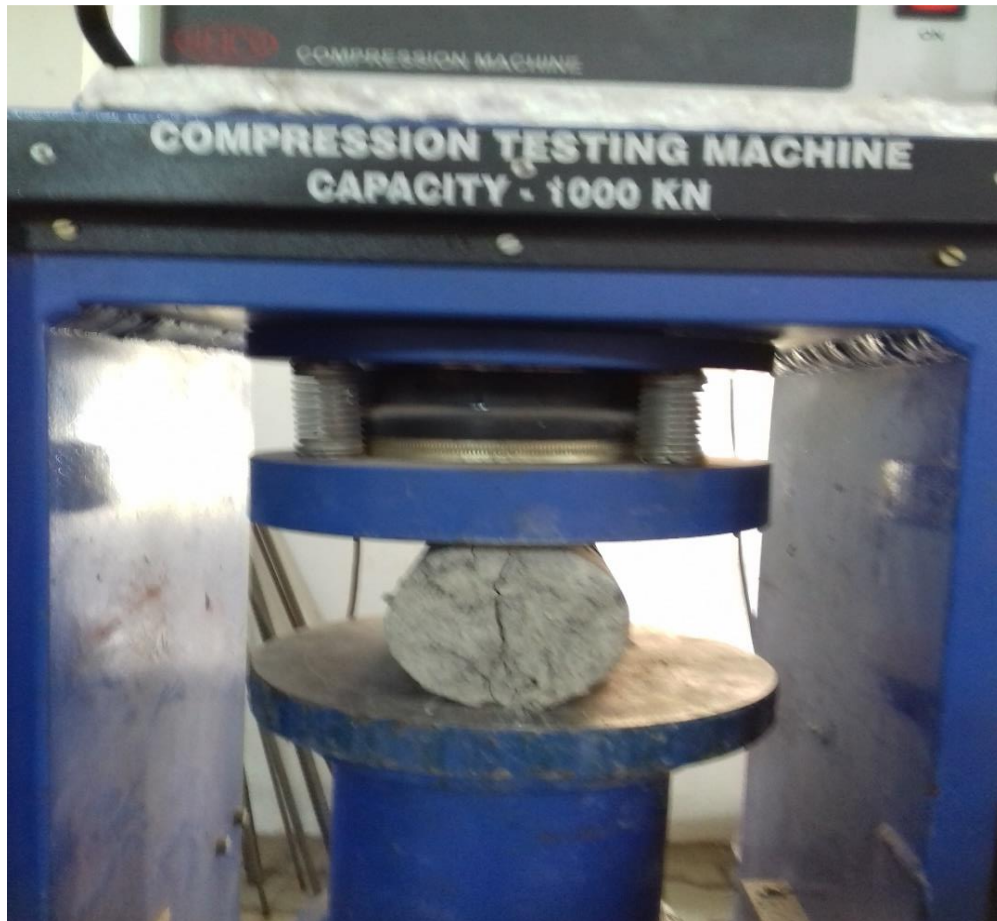
Fig 19: Split-Tensile strength testing alignment
