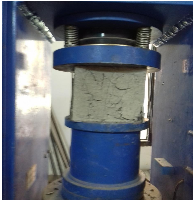
Fig 18: Compressive strength testing
