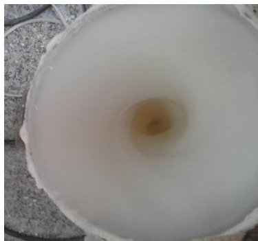
Fig 3.2 sonication of Nano-silica
