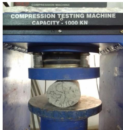
Figure 7.5 showing set up of split tensile test investigation
