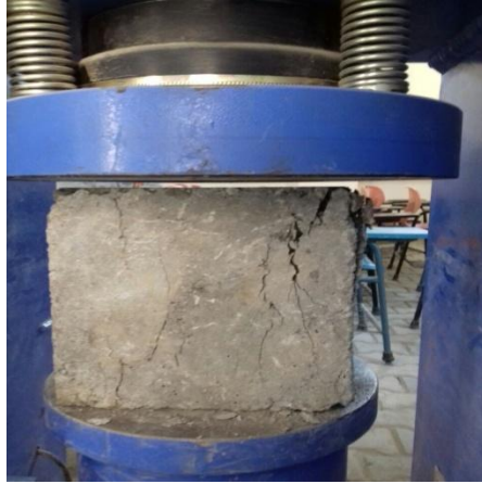
Figure 7.4 showing set up of compressive test investigation
