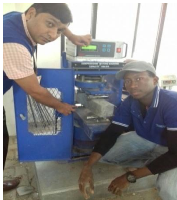
Figure 7.6 showing set up of flexure strength test investigation
