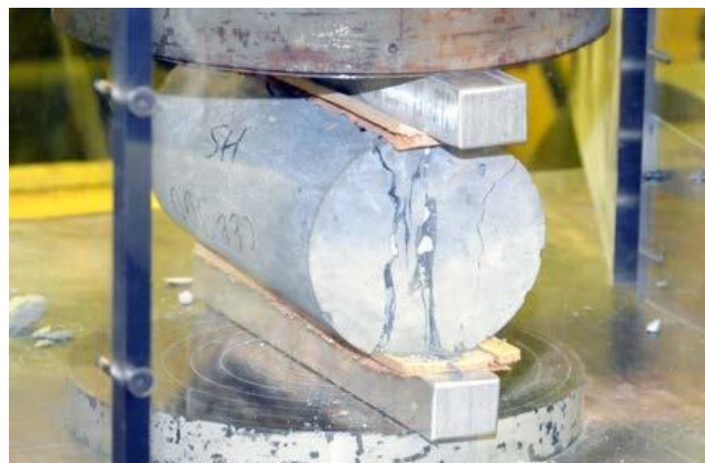
Fig.3 split tensile strength test
