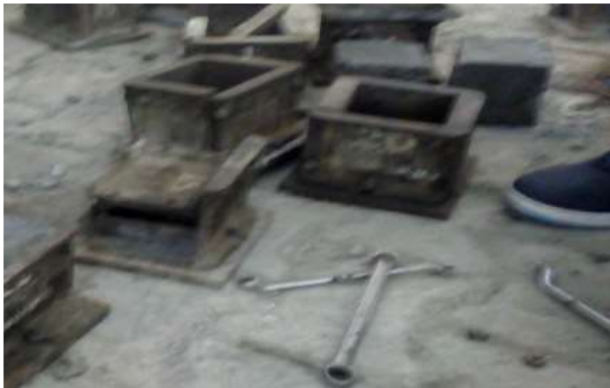
Figure 14 : Preparation of Moulds
