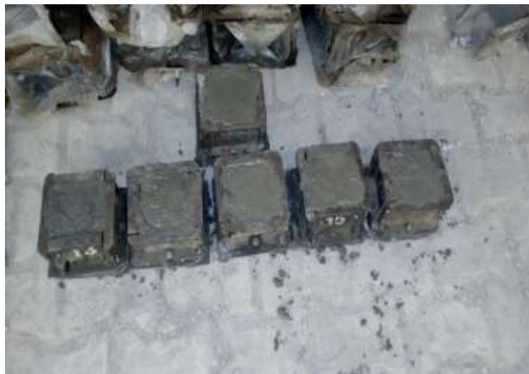
Figure 17 : Curing for 24 hours
