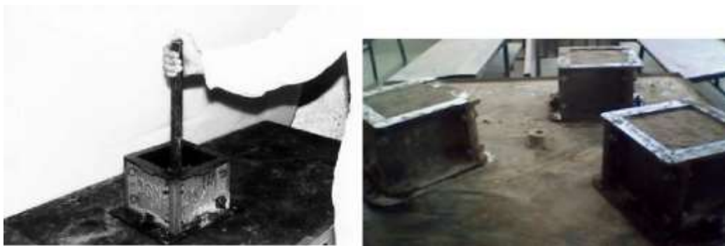
Figure 15 : Compacting of Concrete using Vibratory Table and Tamping Rod
