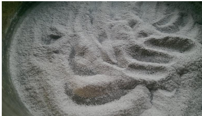
Figure 3.1. Glass powder particle size less than 75 microns
