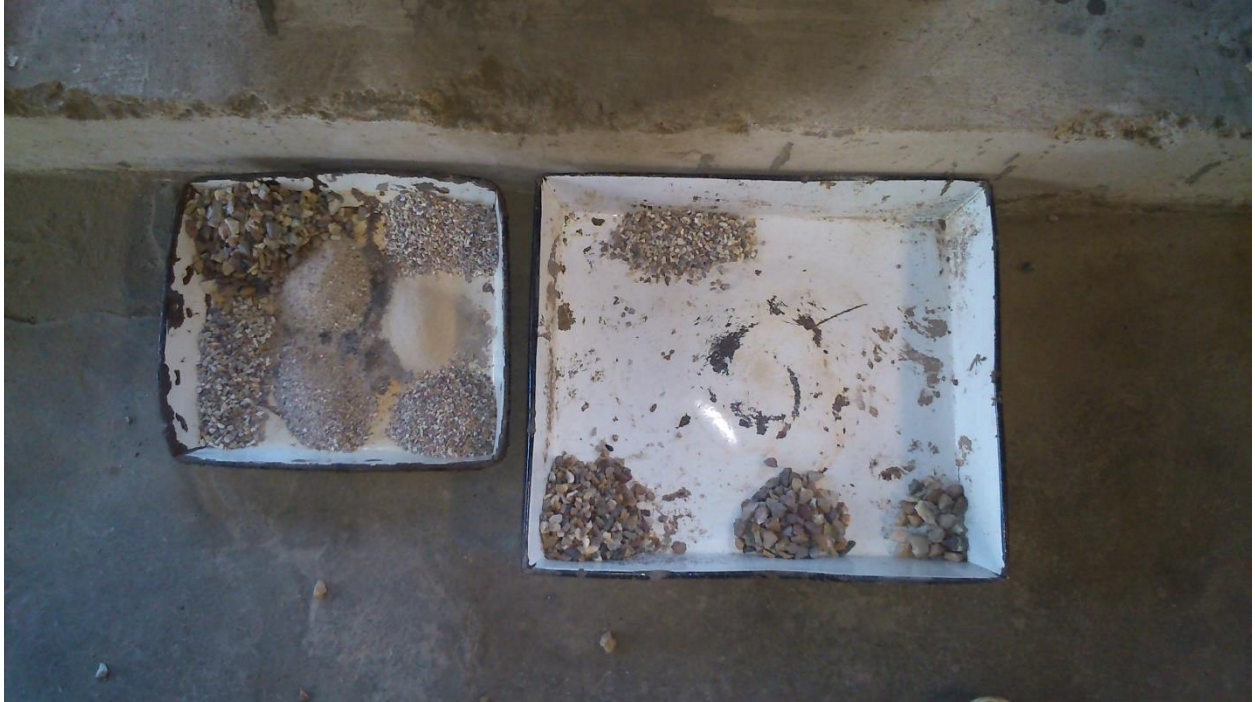
Figure No. Material prepared for Marshall Test
