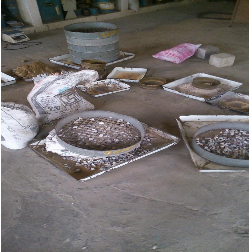
Figure no: Sieve analysis for prepared the Marshall specimen
