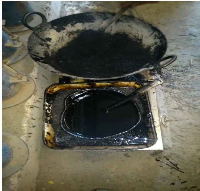
Figure No: Heating the aggregate and bitumen
