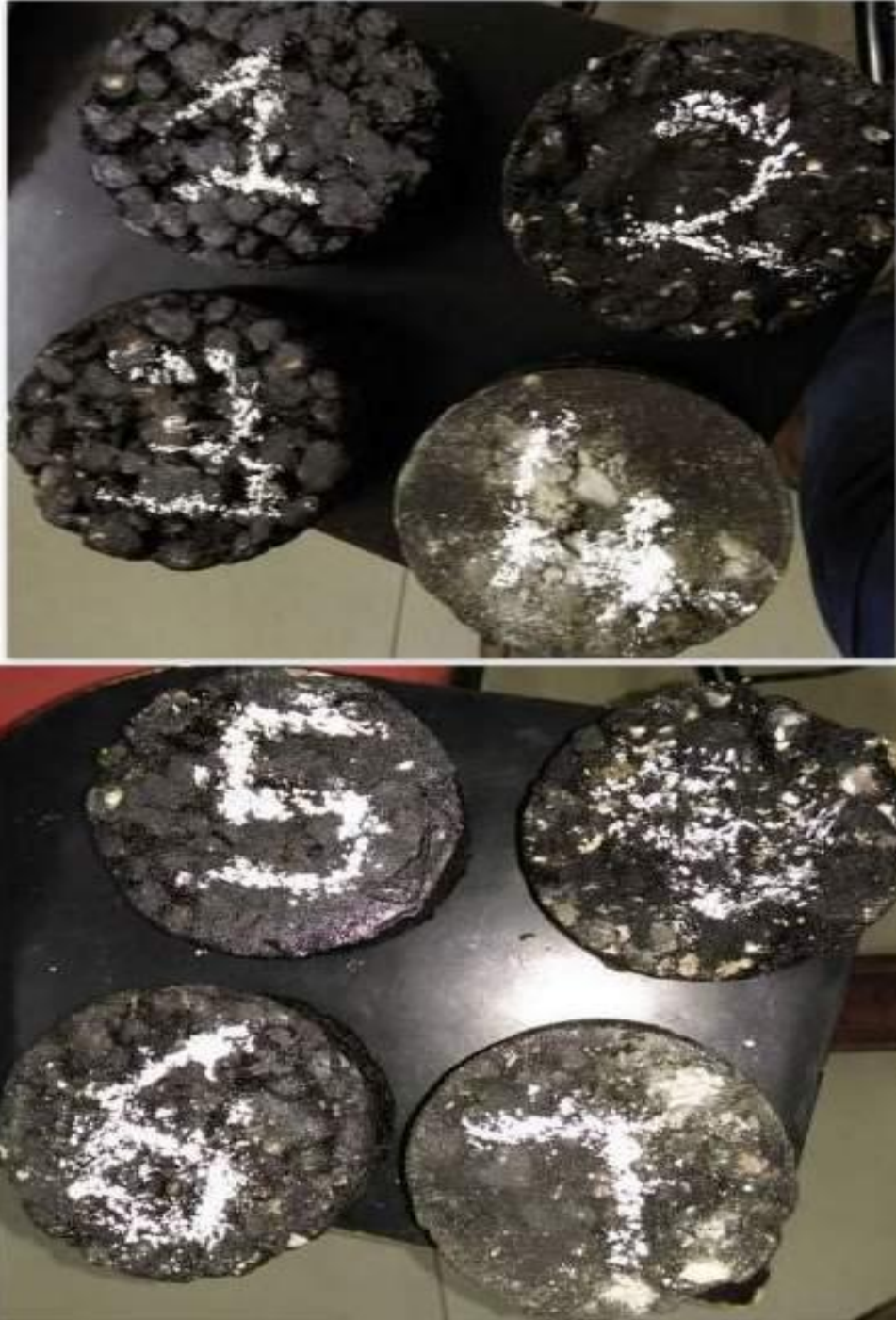
Figure 3.15 : Marshall test specimens
