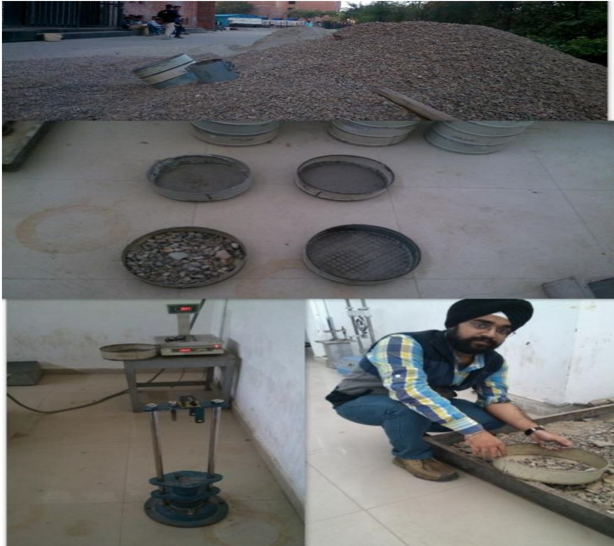
Figure 3.1 : Aggregate sample collection for aggregate impact test
