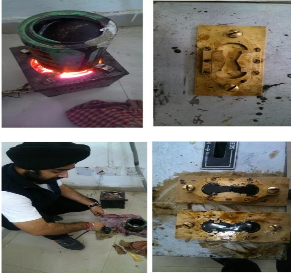
Figure 3.6 : Preparation of bitumen specimen in Briquette Mould along with heating bitumen
