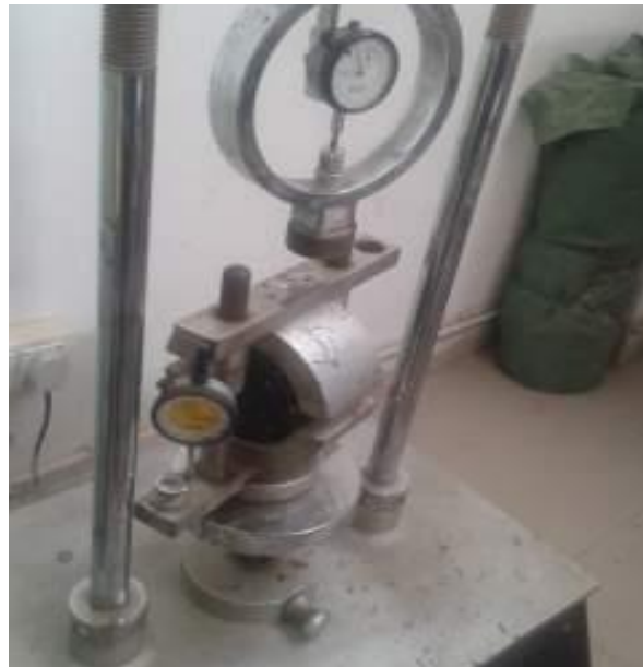
Figure 3.12 : Marshal Stability & Flow Value Test Apparatus
