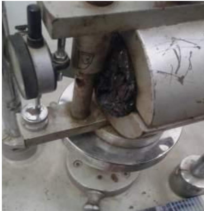
Figure 3.14 : Marshal test specimen after the application of load
