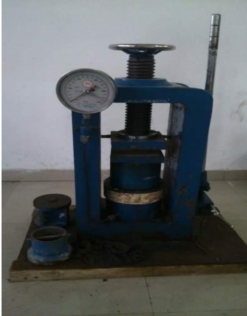
Figure 3.2 : Aggregates “crushing value” test apparatus
