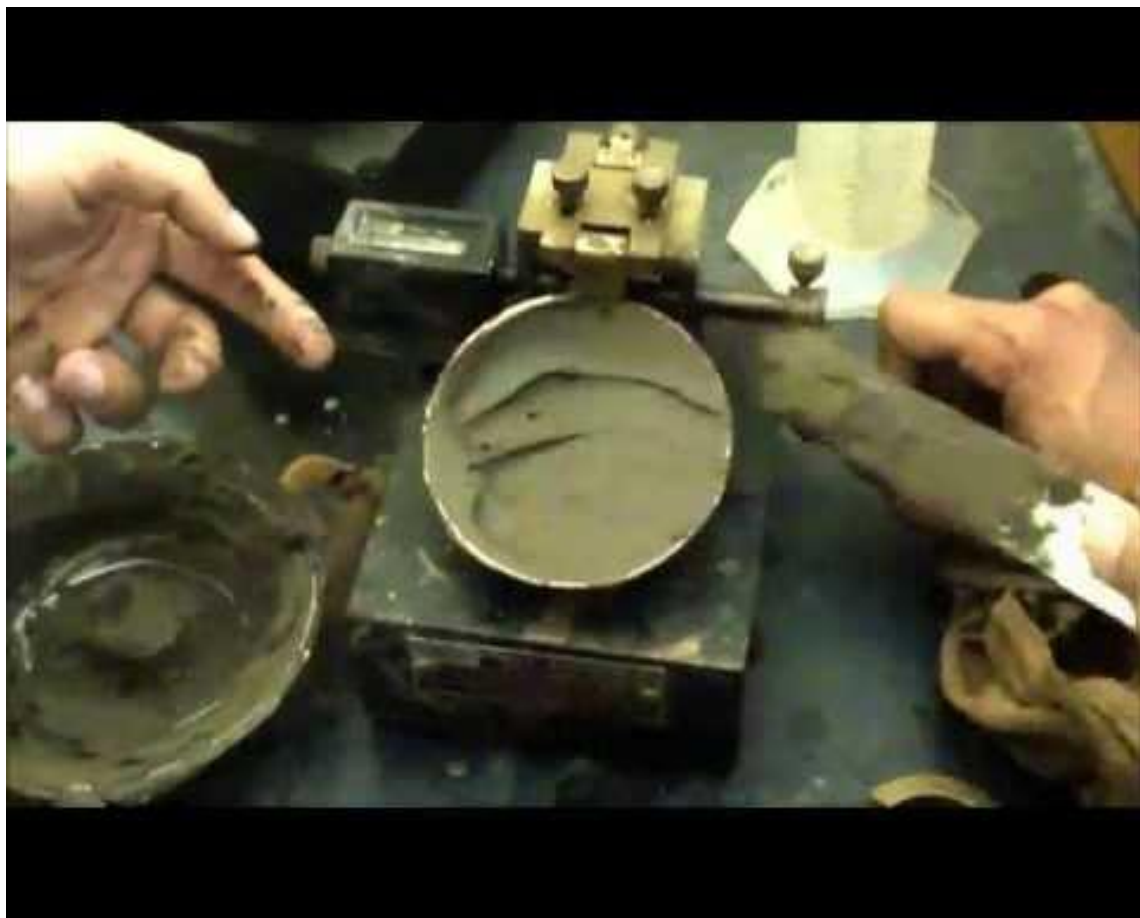
Figure 5.3: Evaluation of Liquid limit by Casagrande's experiment
