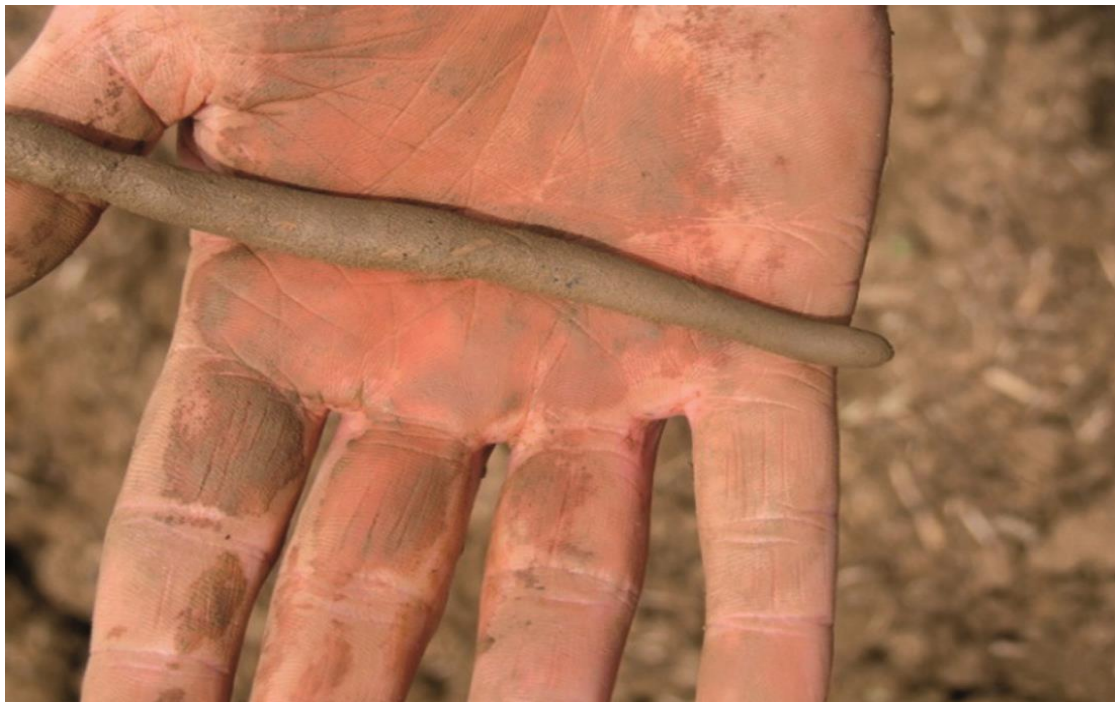
Figure 5.4: Evaluation of Plastic Limit (PL)
