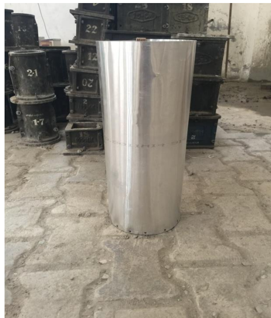
Figure 6.2: Mould for circular column
