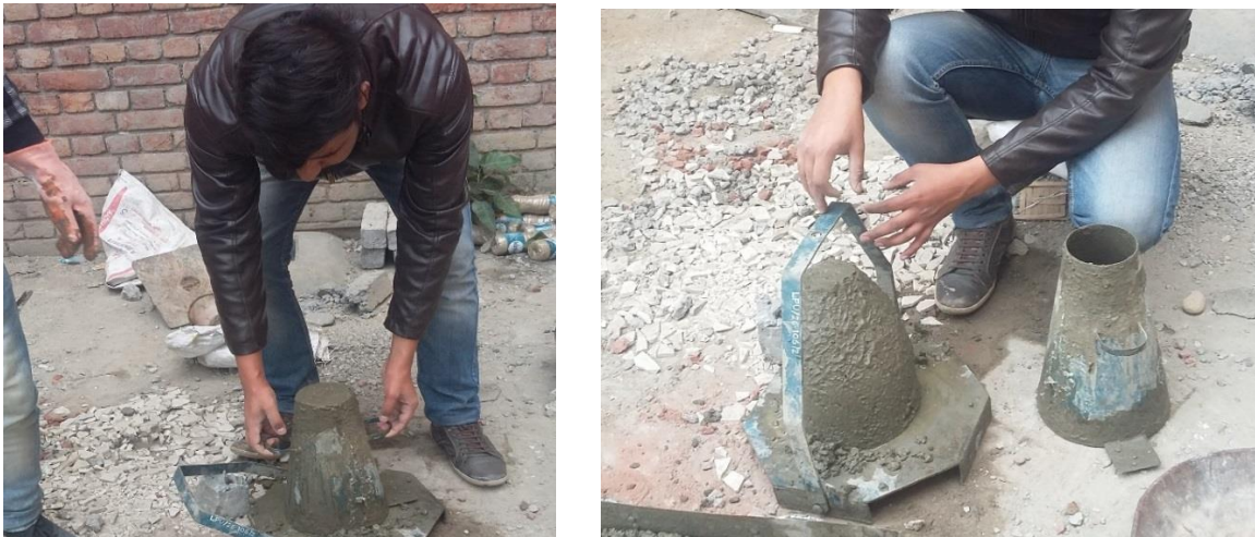
Figure 7.1 Workability test using slump cone
