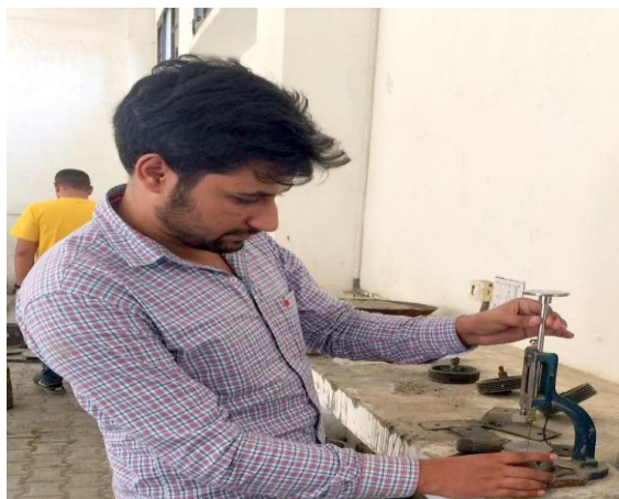
Figure 6.5 Sample under vicat apparatus for IST and FST
