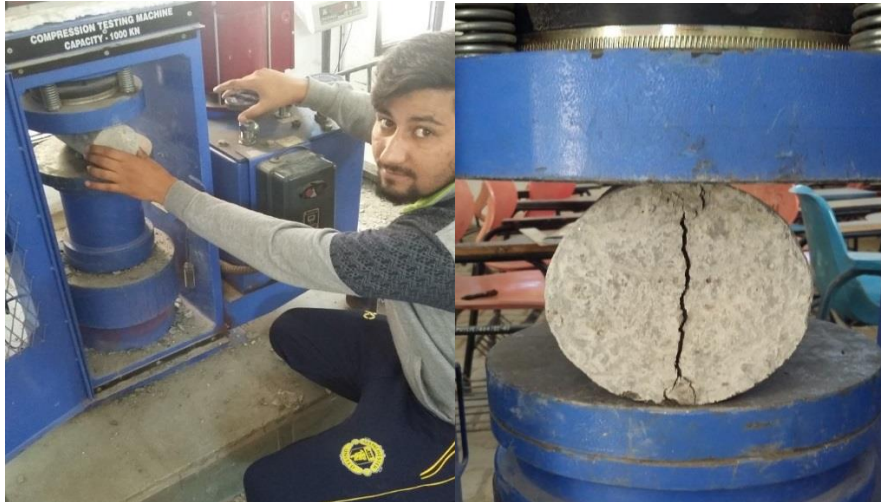
Figure 7.10 Sample during tensile test
