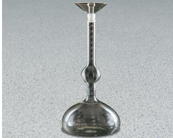
Figure 6.6 Le-chatelier's apparatus for specific gravity test
