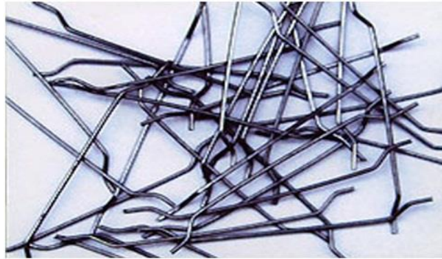
Figure 6.1 Shape of Steel Fibres
