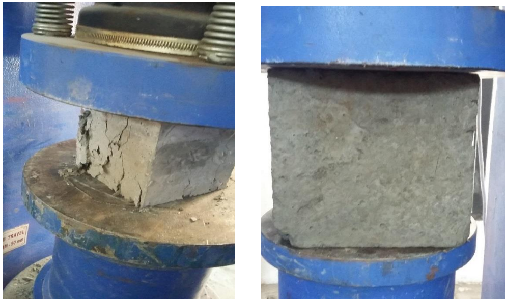
Figure 7.6 Sample under compression testing machine
