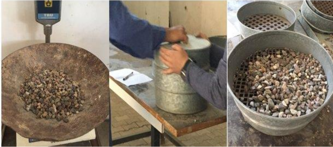
Figure 6.7 Sieving of CA for calculation of fineness
