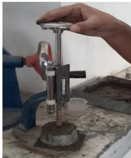
Figure 6.2 Sample under Vicat Apparatus
