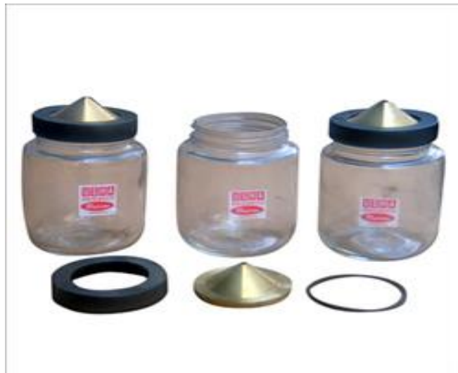
Figure 6.8 Pycnometer used for specific gravity calculation of FA
