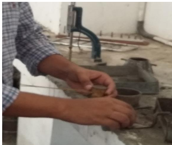
Figure 6.3 Making sample for soundness test
