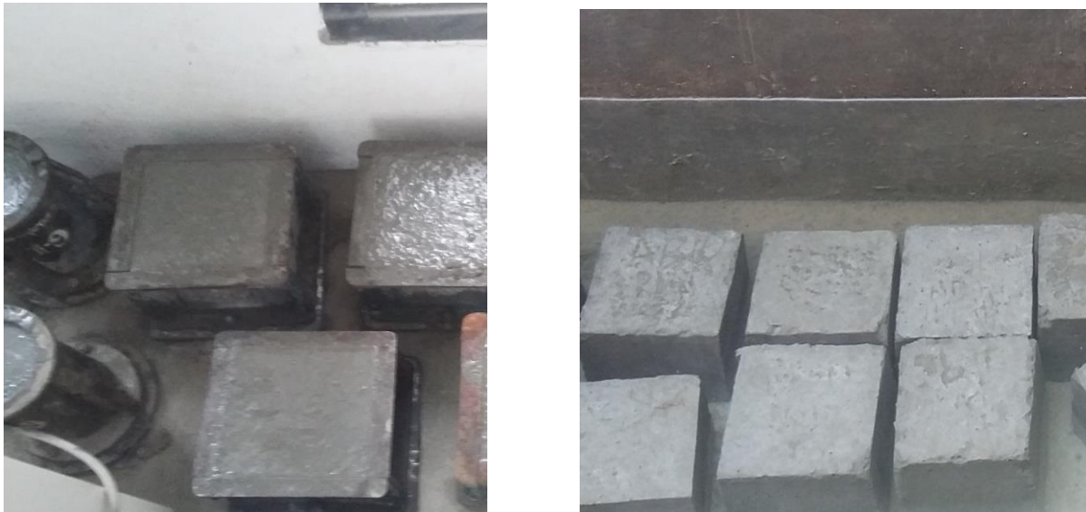
Figure 7.4 Casting and curing of concrete cubes
