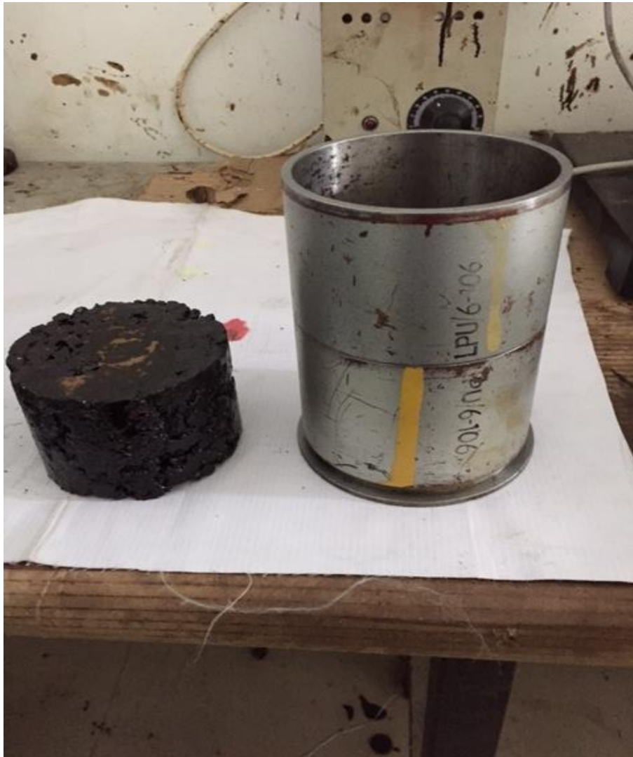
Figure 4.1 showing preheated cylindrical mold with collar and base plate
