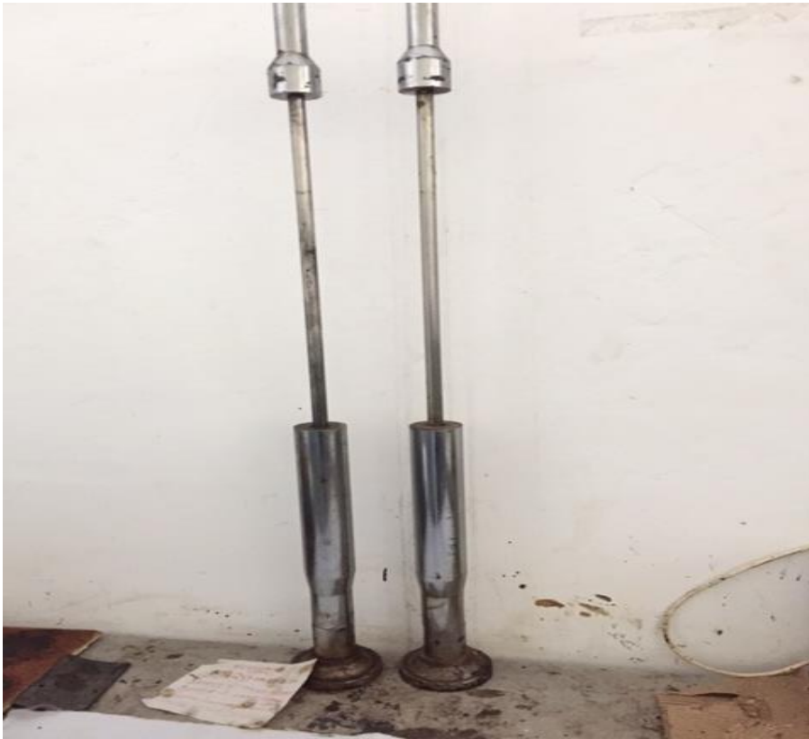
Figure 4.2 showing rammer required for giving blows to the specimen
