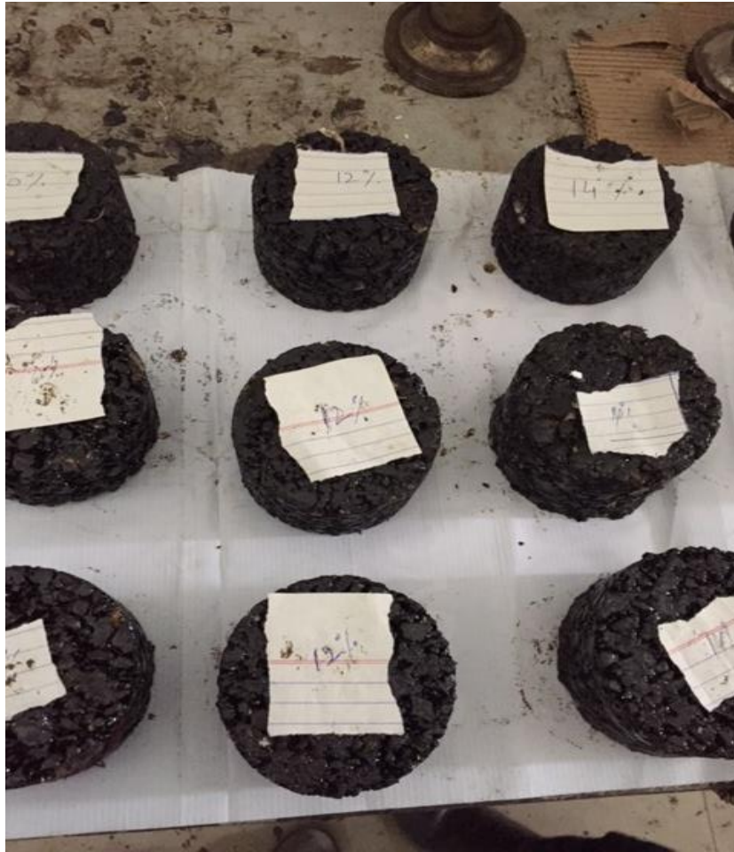
Figure 5.16 showing 12% replacement of bitumen with molasses
