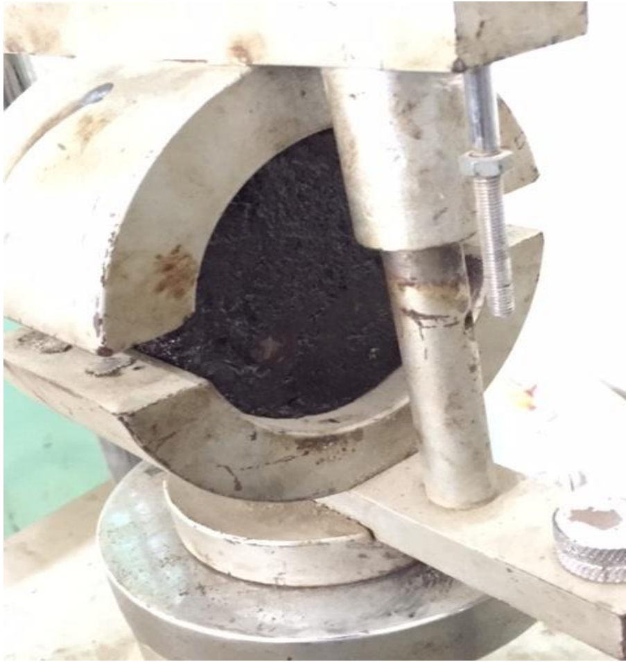
Figure 4.3 breaking head of marshal machine
