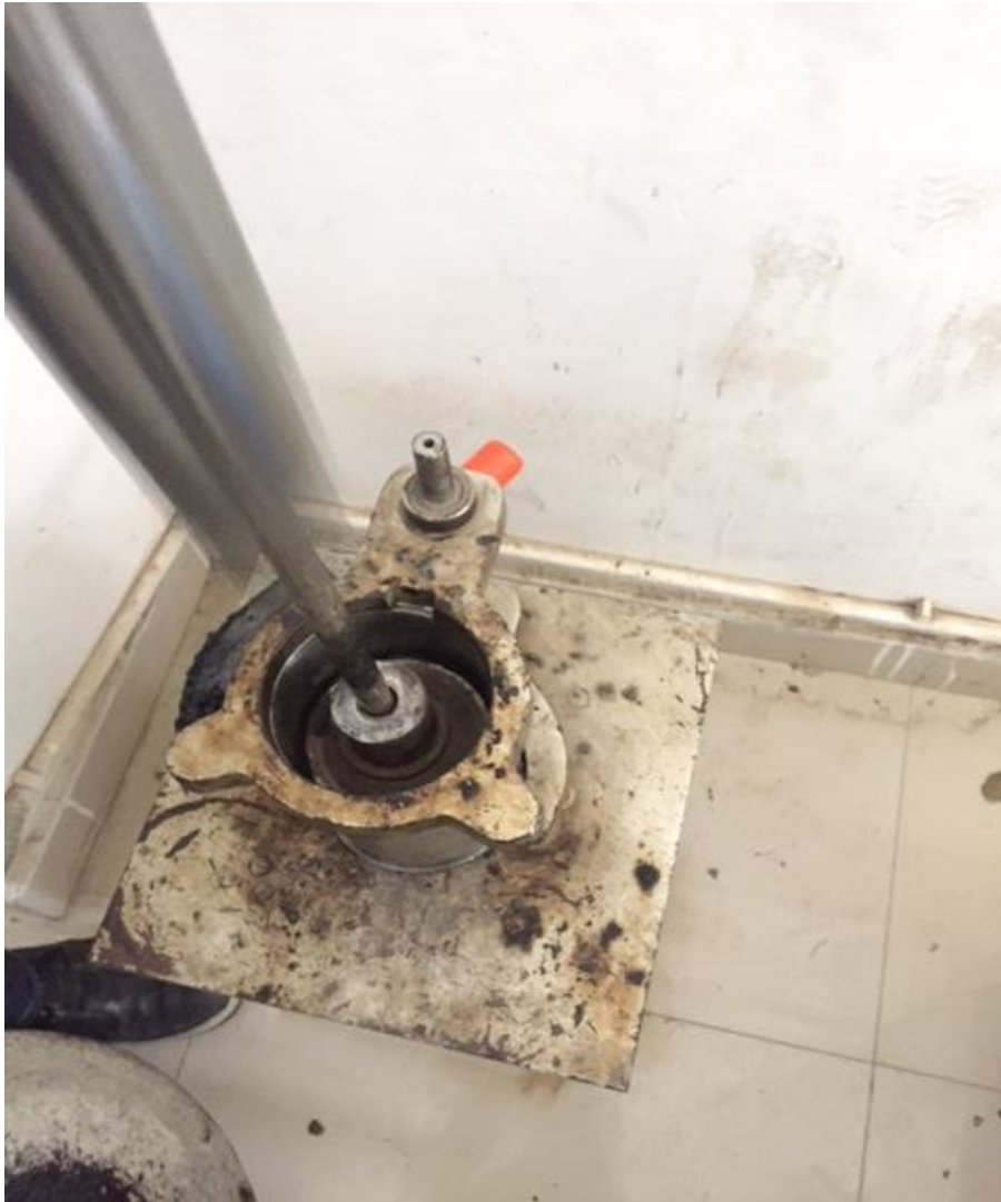
Figure 5.7 Giving blows using hammer (50-60 in 2 minutes)
