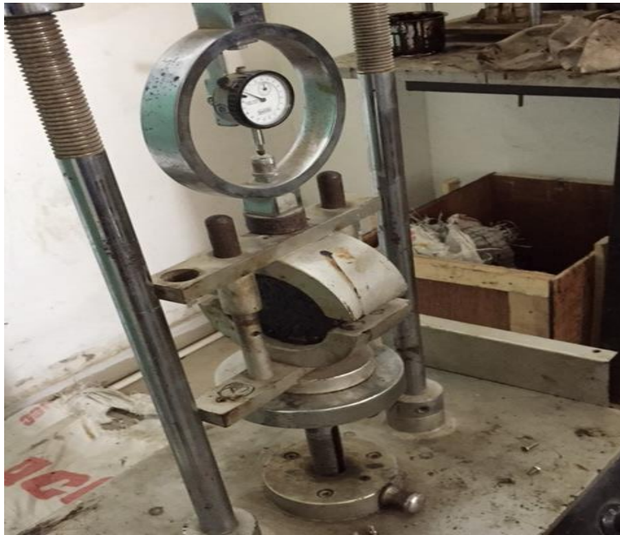
Figure 4.4 Marshal Machine (loading machine)
