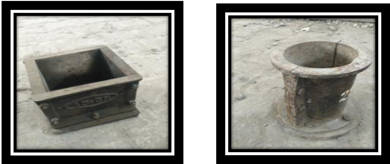
Fig.14 Concrete cube and cylinder mould
