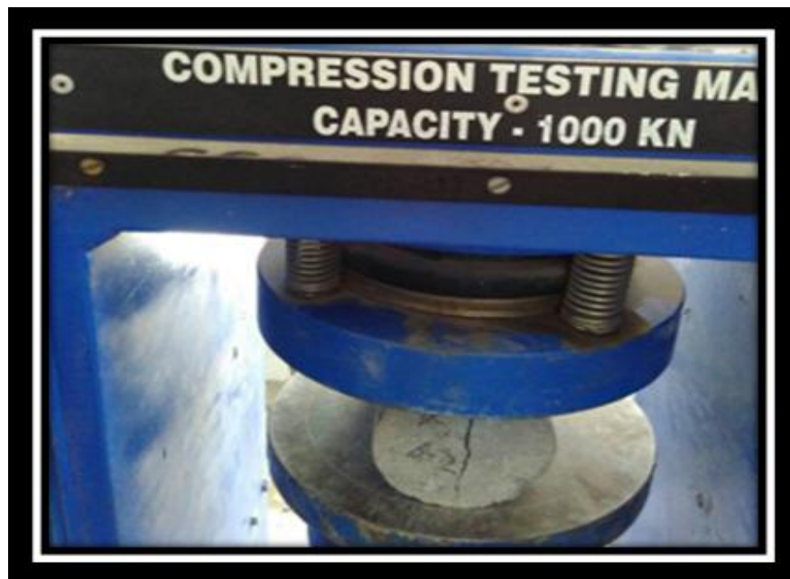
Fig.18 testing of cylinder in compression testing machine
