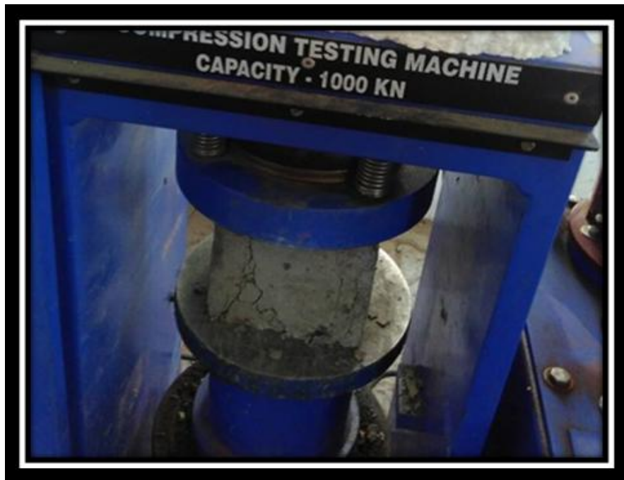
Fig.17 Testing of cube in Compression testing machine
