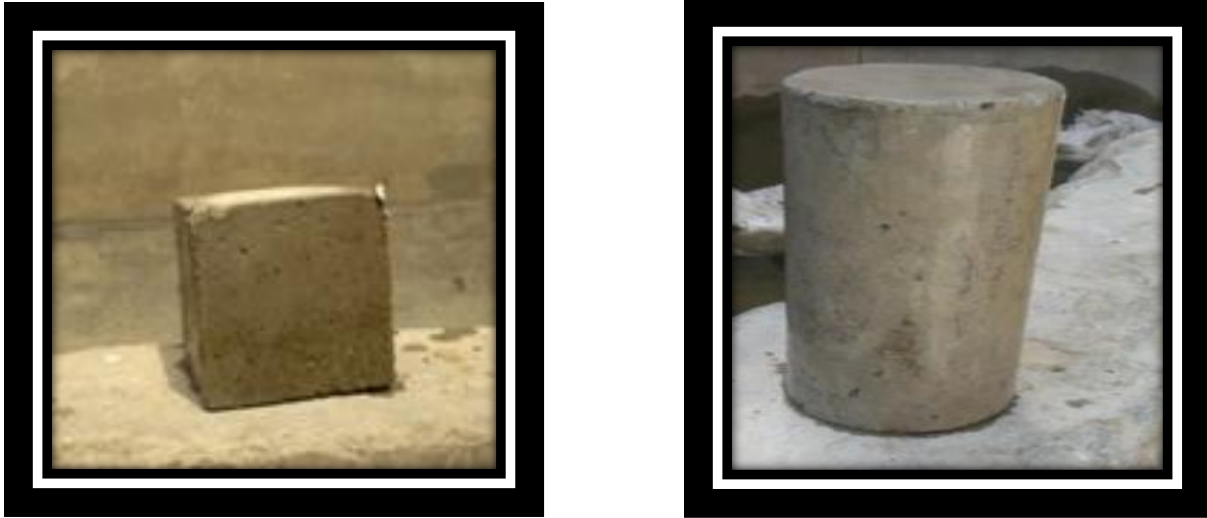
Fig.16 Concrete cube and cylinder after 28 days of curing
