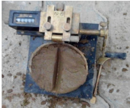
Fig.3.2 Soil Sample with grooving section
