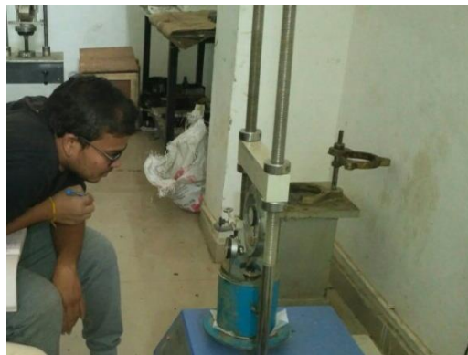
Fig.3.7 observing the CBR test
