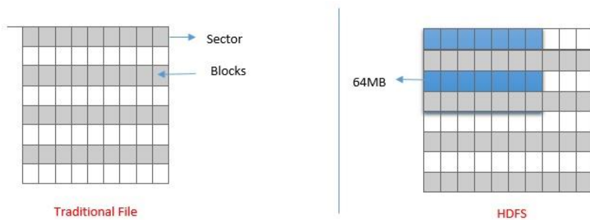
Figure: 1.1 Basic difference between HDFS and Traditional Structure
