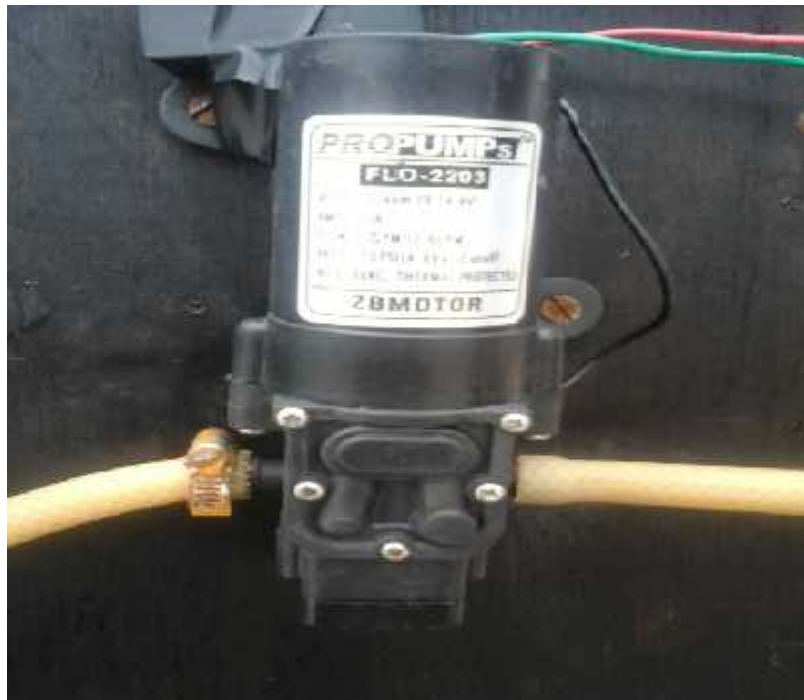
Figure 11: pump used for circulation of water
