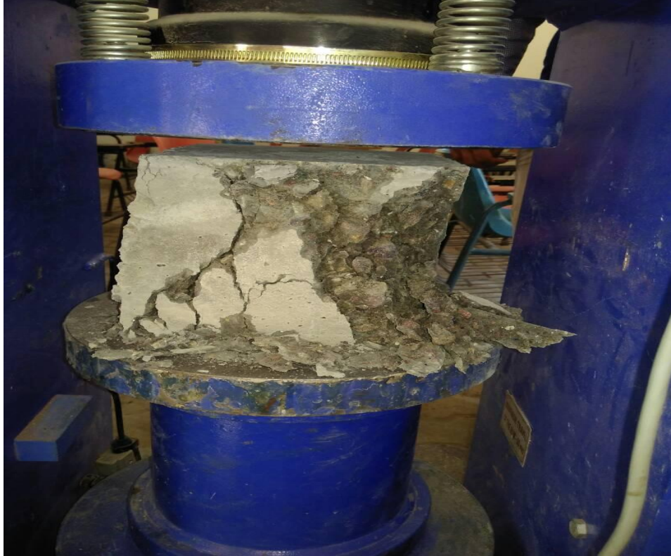
Fig 4.4: Testing of cubes on compression testing machine
