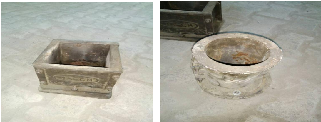
Fig 4.1: Concrete cube and cylinder mould.
