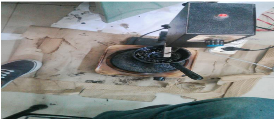
Figure 4.1 Mixing of aged bitumen with WCO (source- During Testing)
