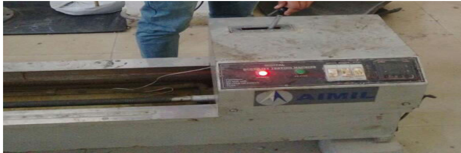
Figure 1.4 Ductility Machine (source- During testing)
