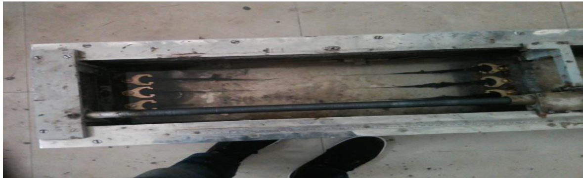
Figure 4.2 Threads of Bitumen in Ductility Machine
