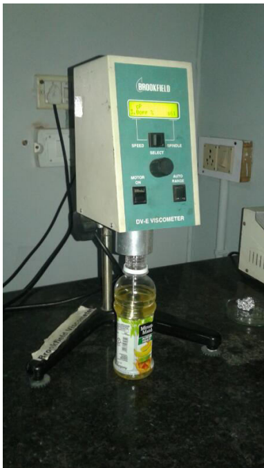
Figure.1.5 Rotational viscometer(Source-During Testing)
