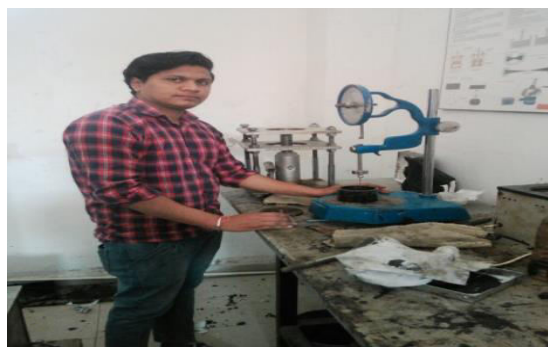
Figure 1.2 Penetrometer for Penetration Test. (Source- During testing)
