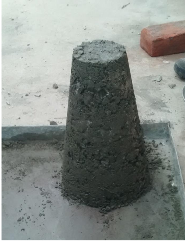
Figure 7.1: Rubberized concrete sample for workability test
