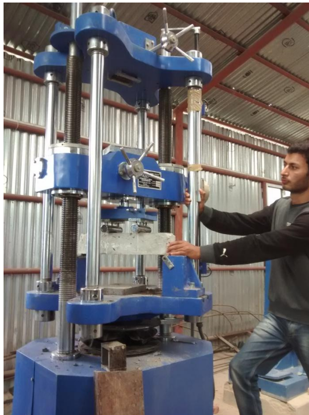
Figure 7.6: Two point flexural loading on beam
