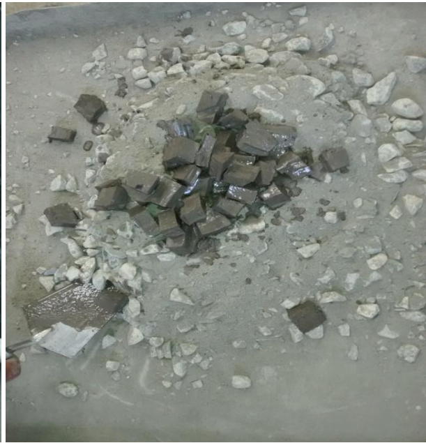
Figure 6.2: Cement paste-treated rubber
