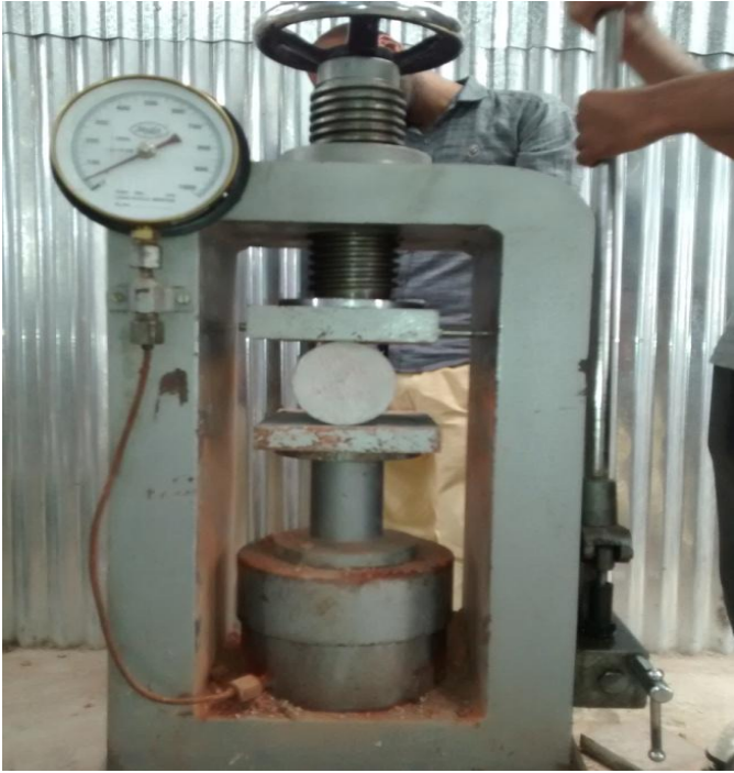
Figure 7.8: cylinder under split tensile load
