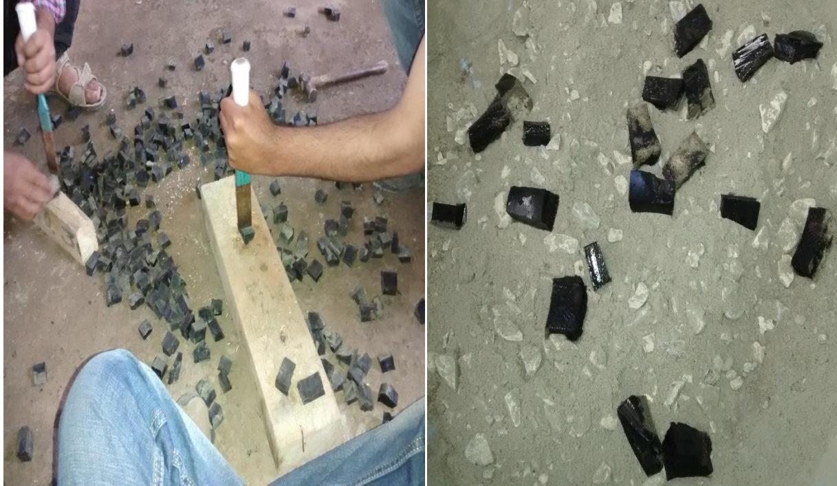
Figure 5.6: Manual cutting of tyre rubber to the size of coarse aggregates
