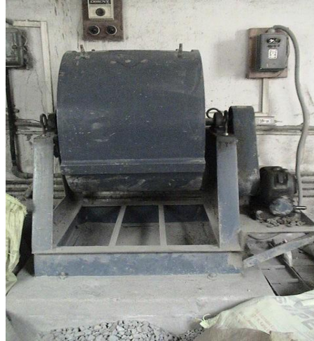
Figure 5.2: Setup for Los Angeles abrasion test
