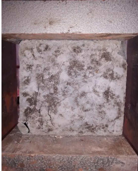
Figure 7.3: Cube under compression
