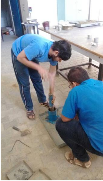
Fig 3.6 tamping soil sample
