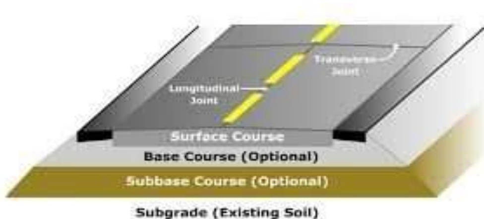
FIGURE 1.1: Road Pavement layers
