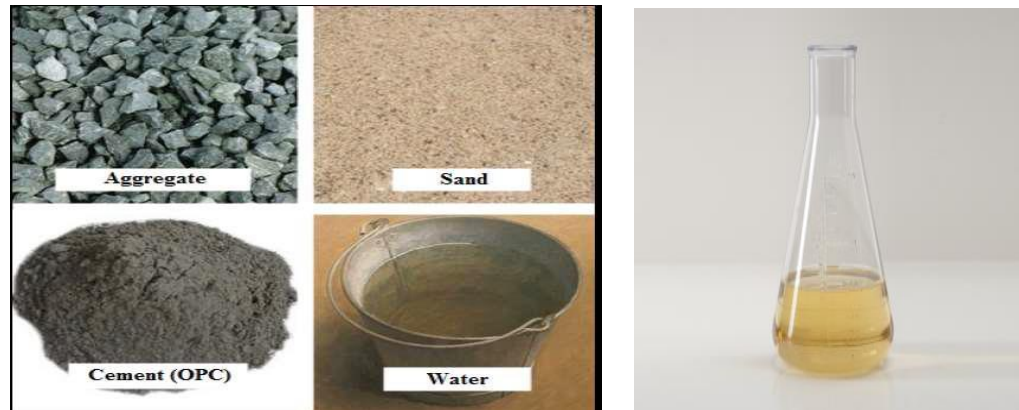
Fig 4.1: Picture of materials used (aggregate, sand, cement, water, microbe)
