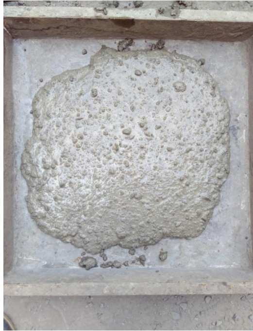
Fig 1.2 Self Compacting Concrete
