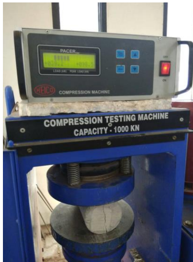
Fig 4.2 Split Tensile Strength test of cylinder
