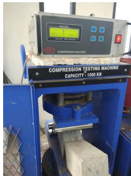
Fig 4.3 Flexural Strength test of beam
