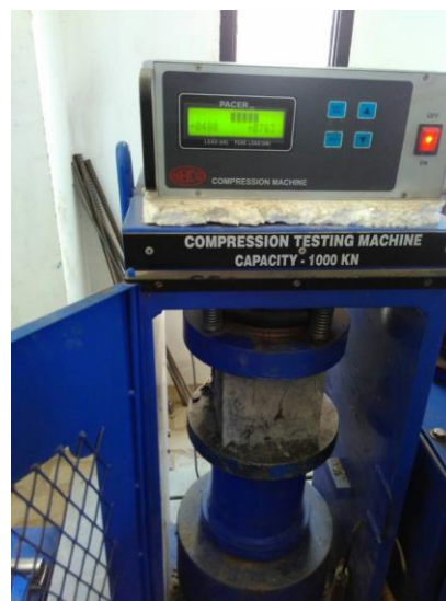
Fig 4.1 Compressive Strength test of Cube
