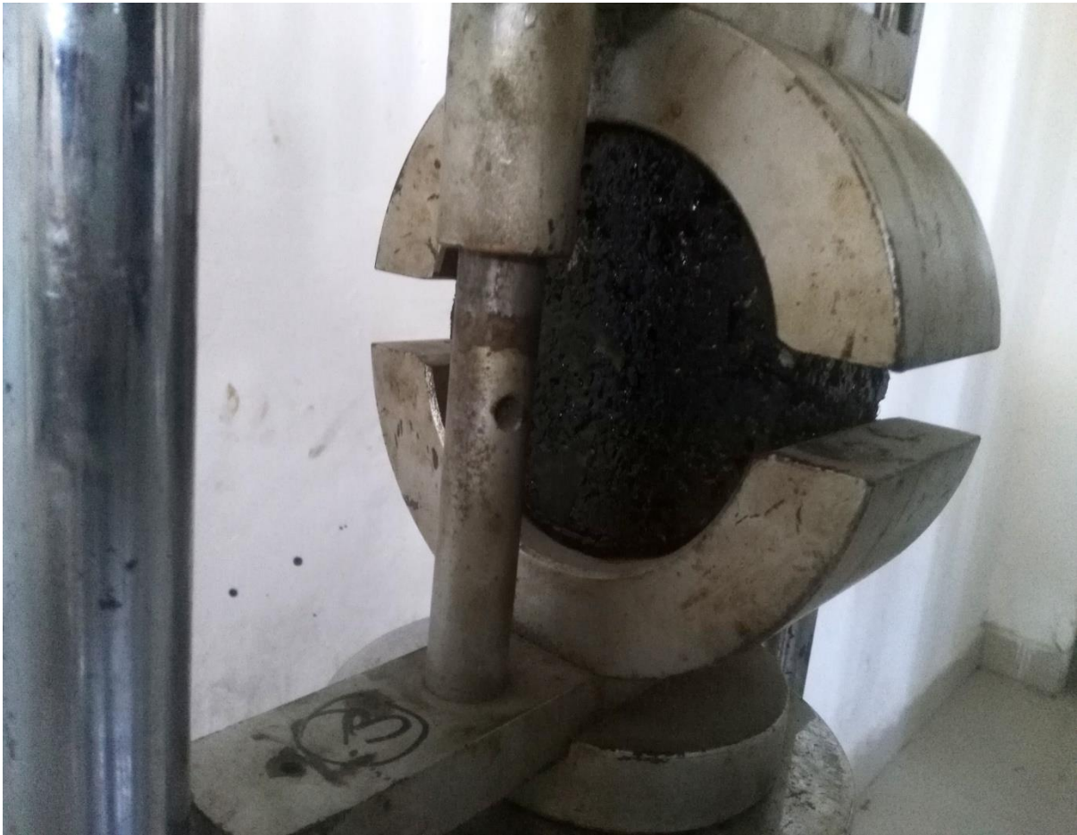
Fig.3.13: Breaking head with sample
