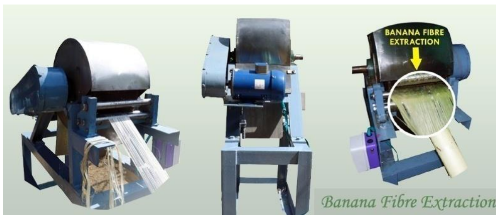
Fig 3.3 Banana fiber extractor
