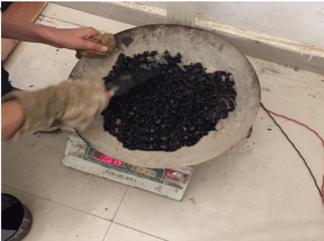
Fig.3.7: Mixing of materials
