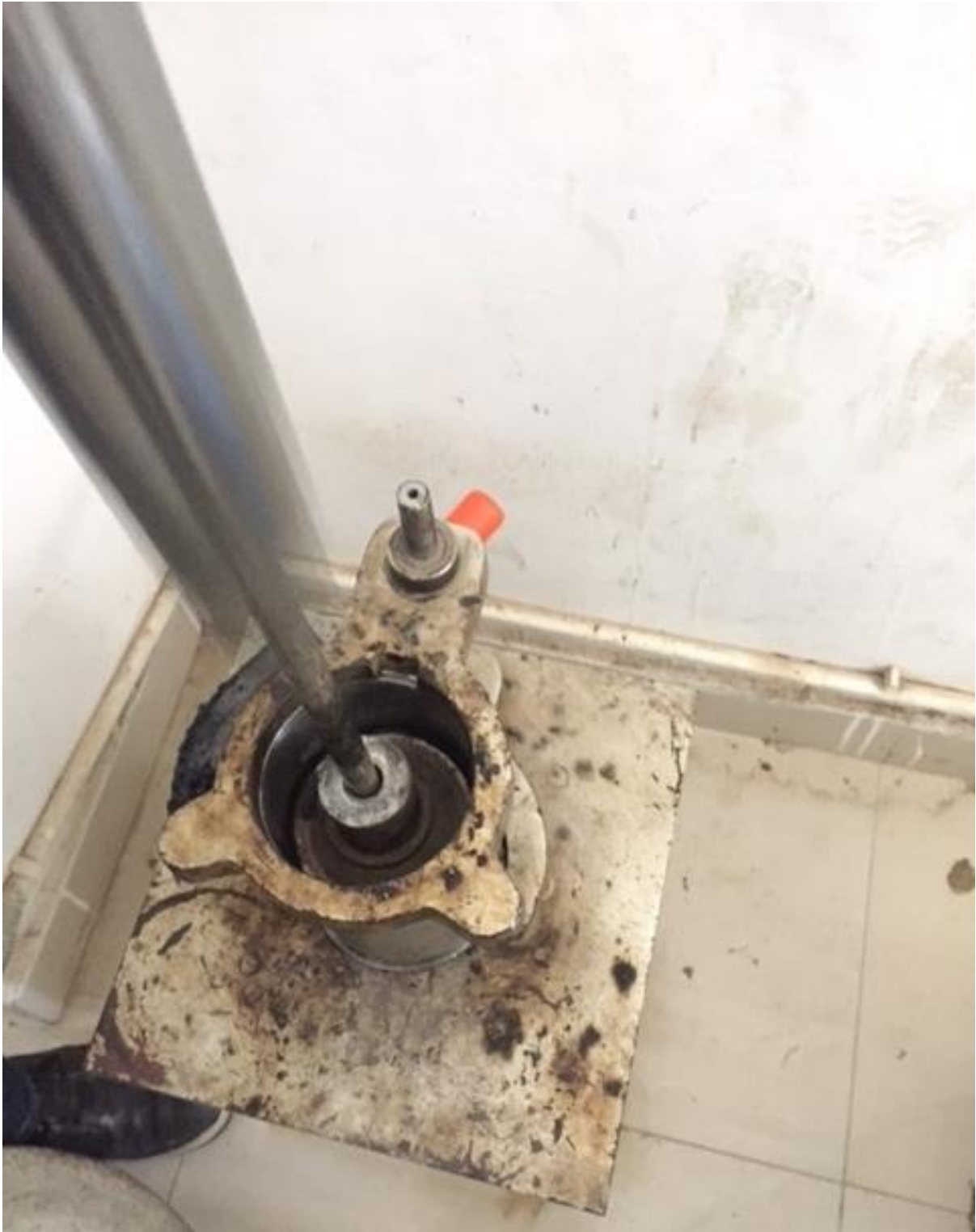
Fig.3.10: Compaction of sample by hammering
