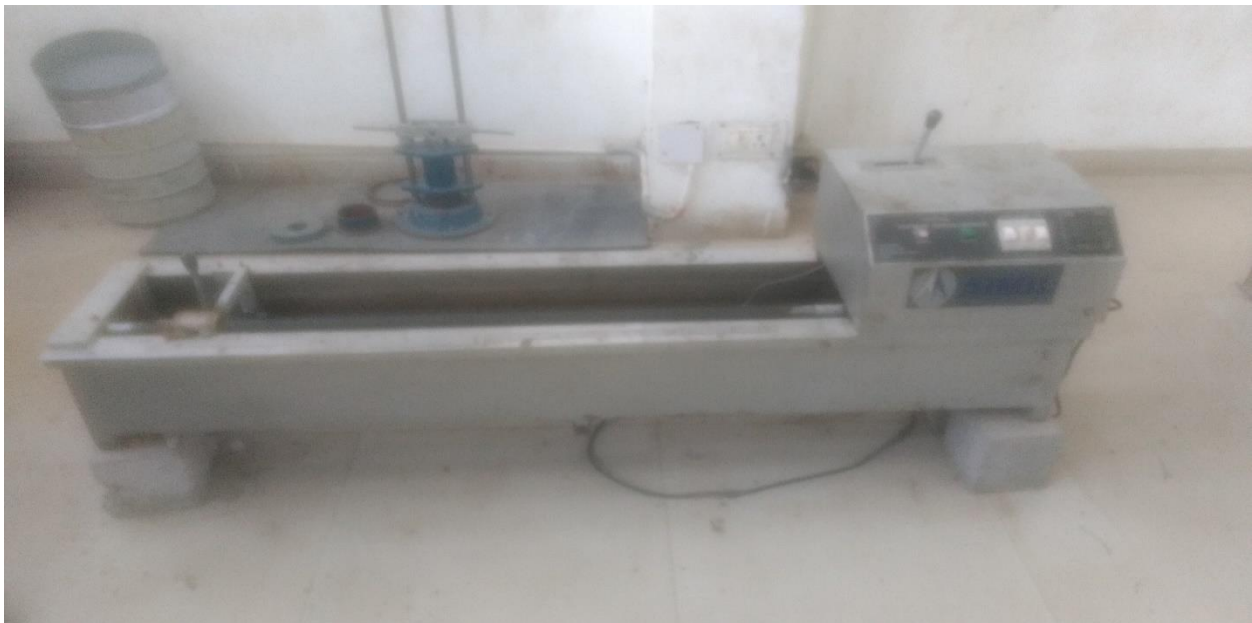
Figure 4.3 – Ductility Testing Machine
