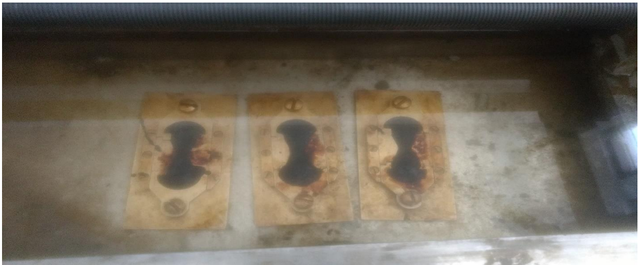
Figure 4.4 – Mold made of brass
