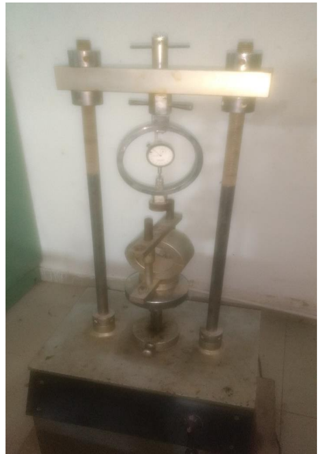
Figure 4.6 – Marshall Stability Apparatus
