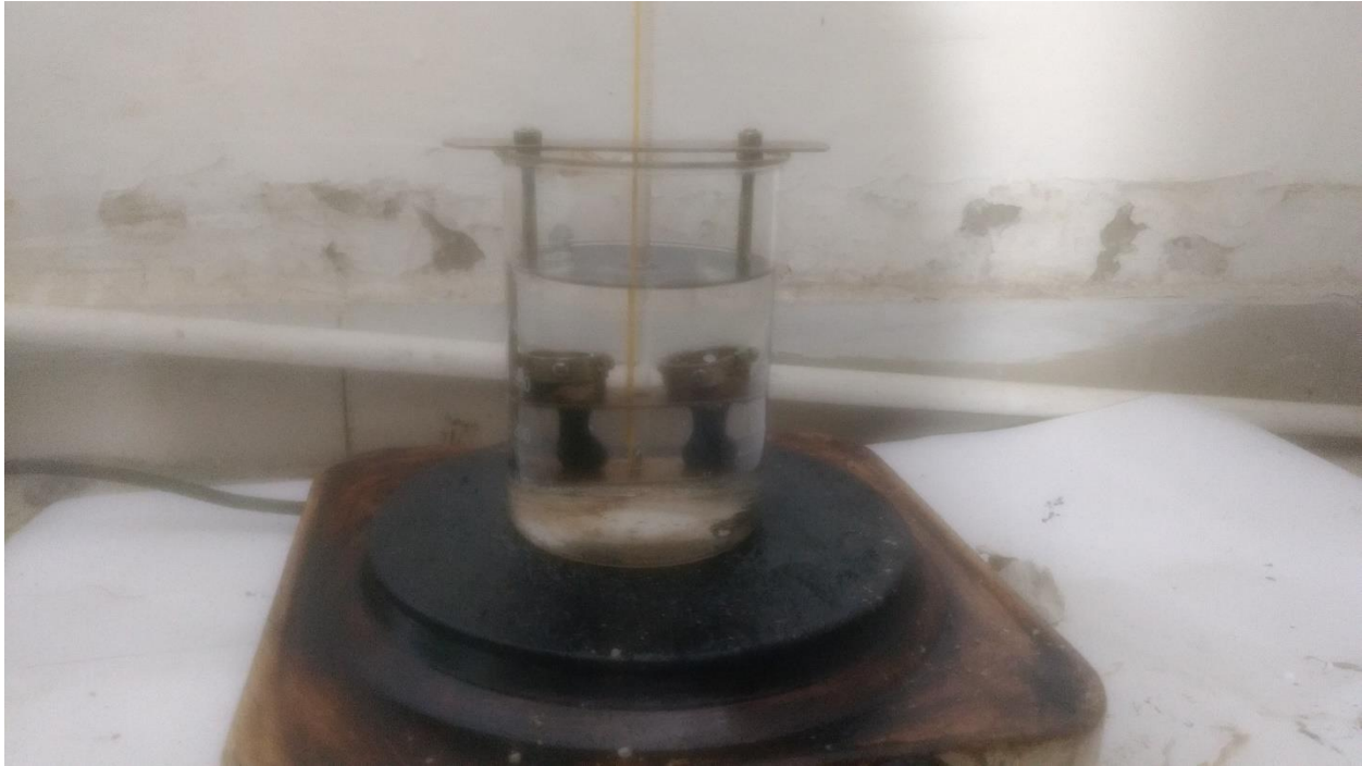
Figure 4.5 –Test Setup for softening point
