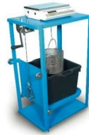
Figure 4.5 Water absorption test
