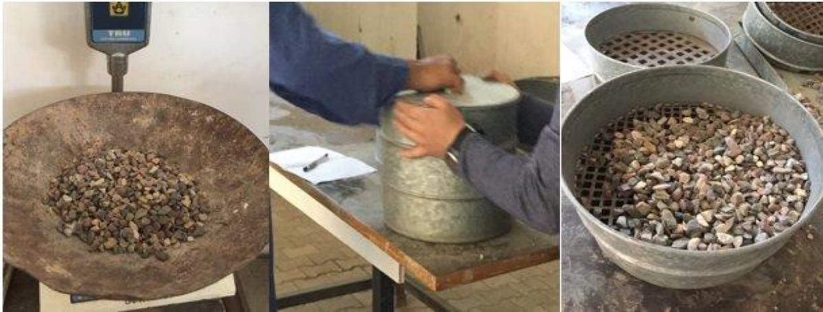
Figure 12: coarse aggregate test
