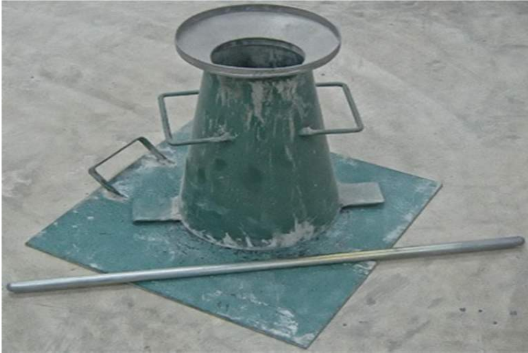
Fig-6:- Showing apparatus for Slump test.
