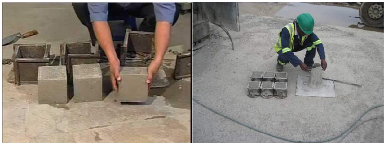
Fig-5 :- showing preparation of concrete cubes for testing.
