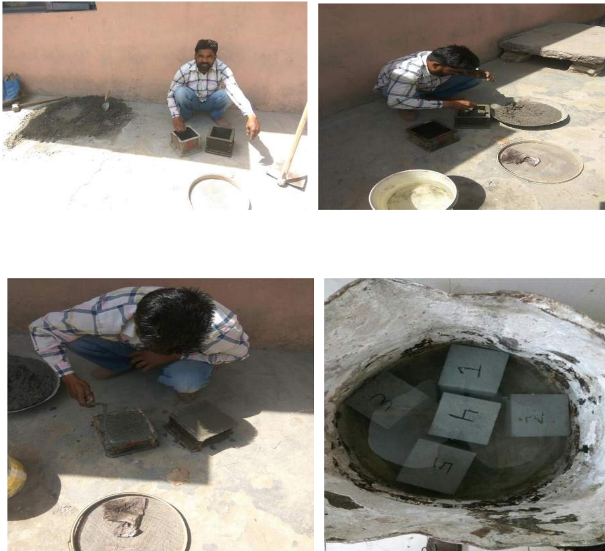
Figure 19:-Pictures taken at the time of Casting Concrete cubes with different Ratios of Treated Waste Water with Potable Water are shown below:-
