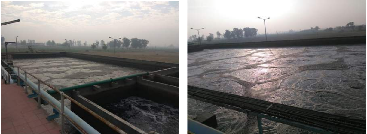
Fig-2 :- STP basin in which aeration and filling is going on
