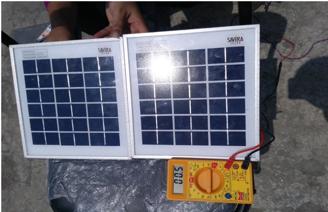
Fig. no. 5.11 Measurement of current with two 6 watt solar panels in 56 Block
