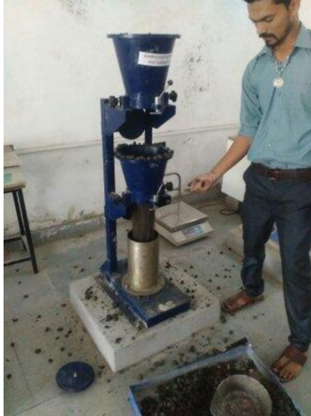
Fig. 6.2: Compacting Factor Test Performance
