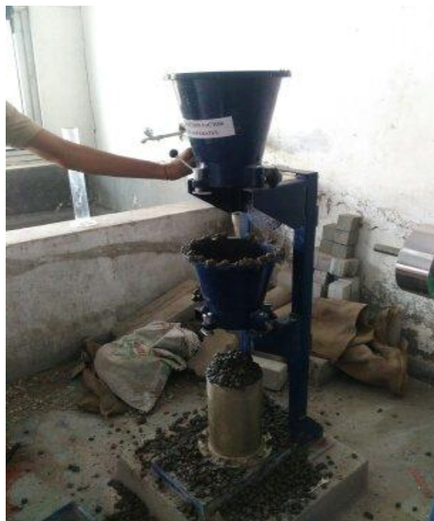
Fig. 5.6: Compacting factor apparatus
