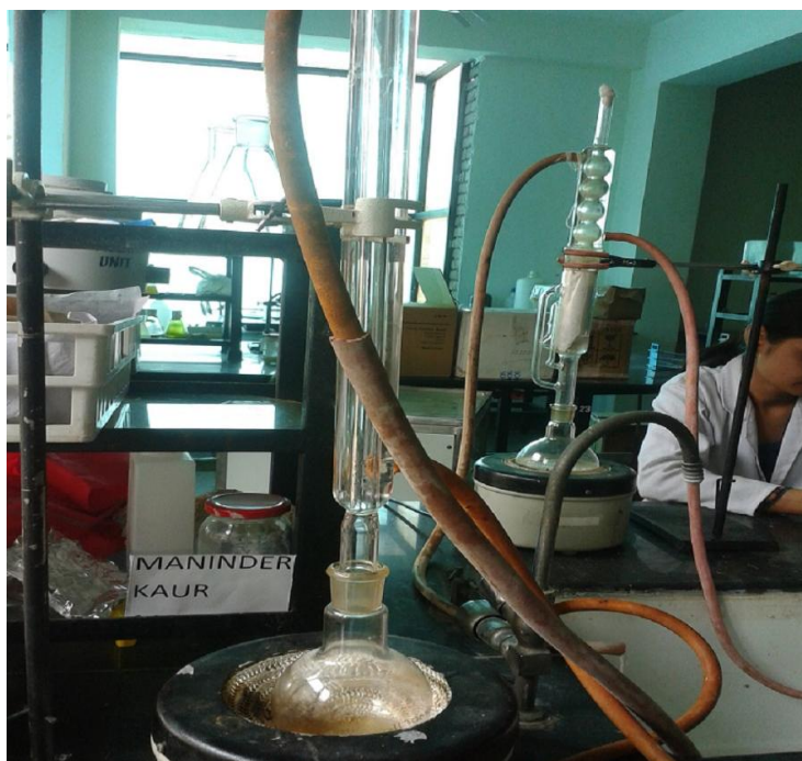
Fig 8:- Tranesterification – Oil sample kept for reflux
