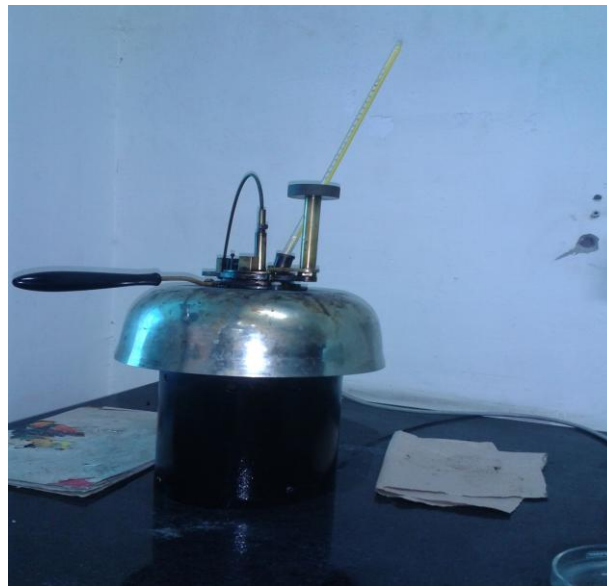
Fig 10:- Pensky Martin apparatus used for the determination of fire point and flash point
