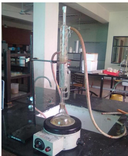
Fig 5:- Extraction of oil using soxhlet apparatus
