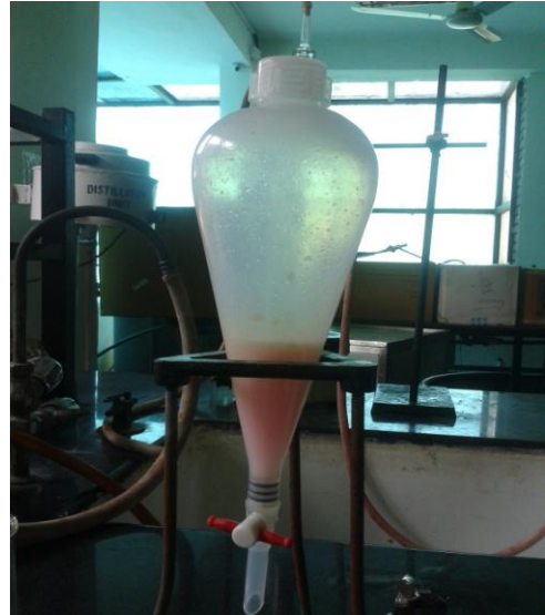
Fig b:- Methyl red indicator is added and 50% H 2 SO 4 is added which gives pink color
