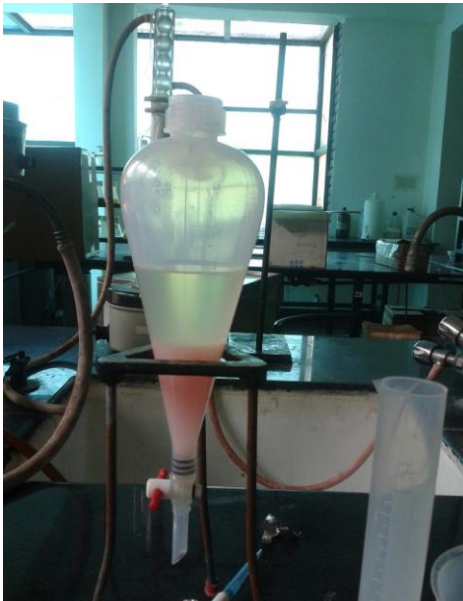
Fig c:- 100 ml petroleum ether is added and shaken which form two layers. Lower layer contain glycerin and upper layer contain biodiesel.
