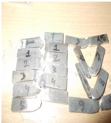
Figure 3.17. (a) Specimens after sensitization and tensile test. (b) Specimens after impact test. (c) Specimens after hardness and microstructure test.
