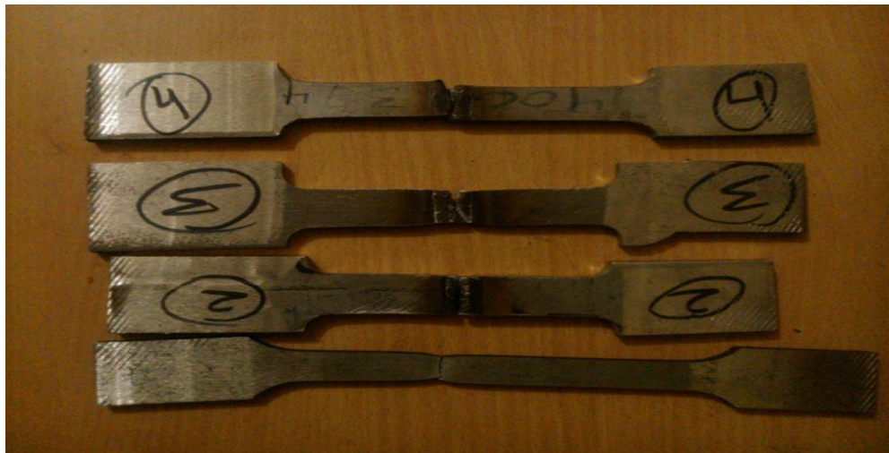
Figure 3.11 Photograph of base metal and as welded tensile tested specimens showing location of fracture.
