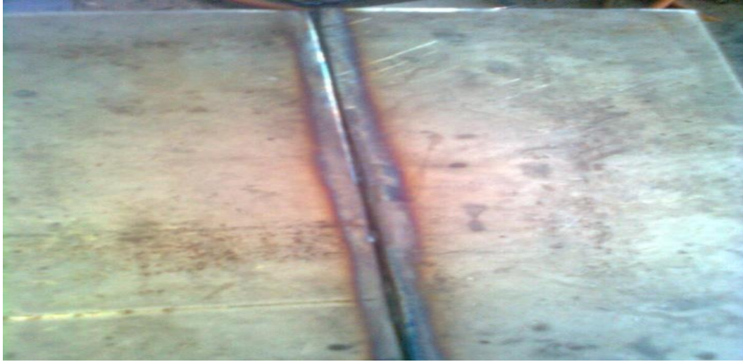
Figure 3.7 Photograph of the sample prior to 2 nd pass.
