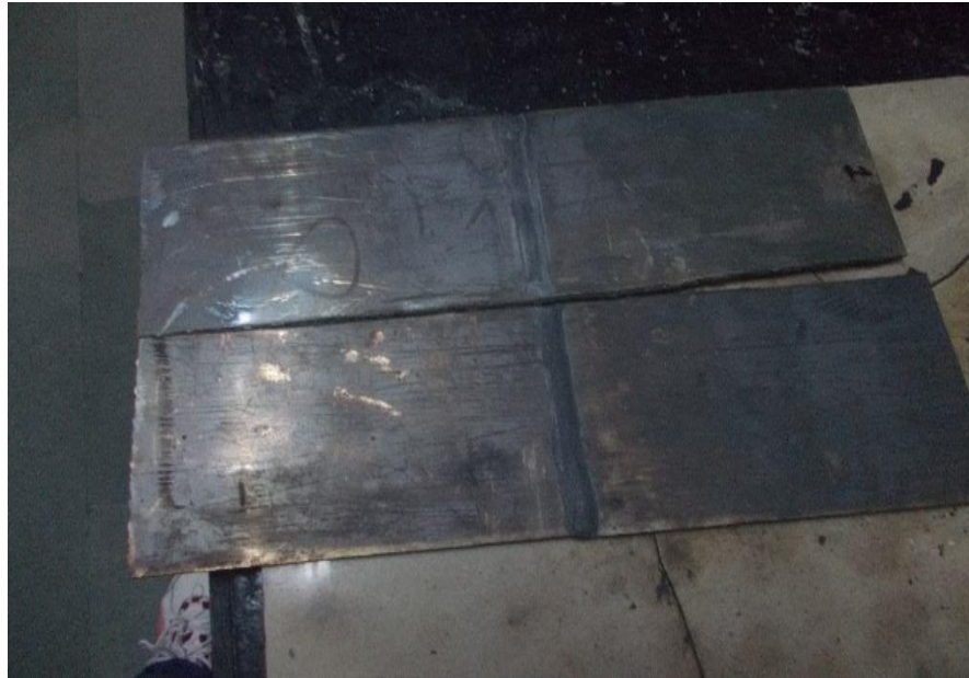
Figure 3.15. Photograph showing the base plates in welded condition for sensitization studies.
