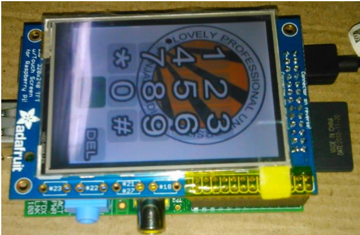
Fig 25: Python based number dialer on Raspberry pi
