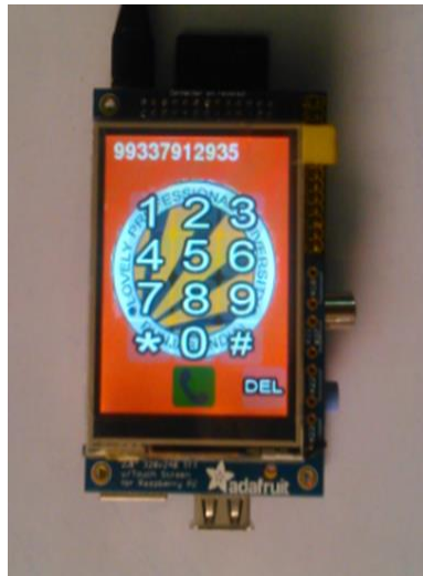
Fig 26: Number dialer pad (using python GUI)
