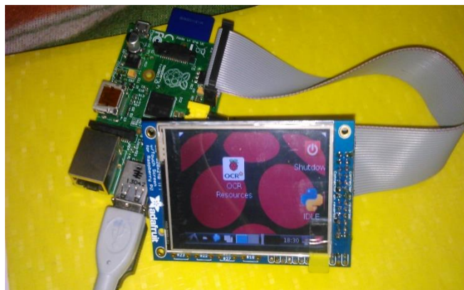
Fig 24: Pi TFT 2.8” interface with Raspberry pi from Adafruit
