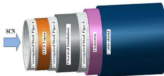
Figure 3-1 Geometry of HTS coaxial cable with different insulations modelled using ABAQUS
