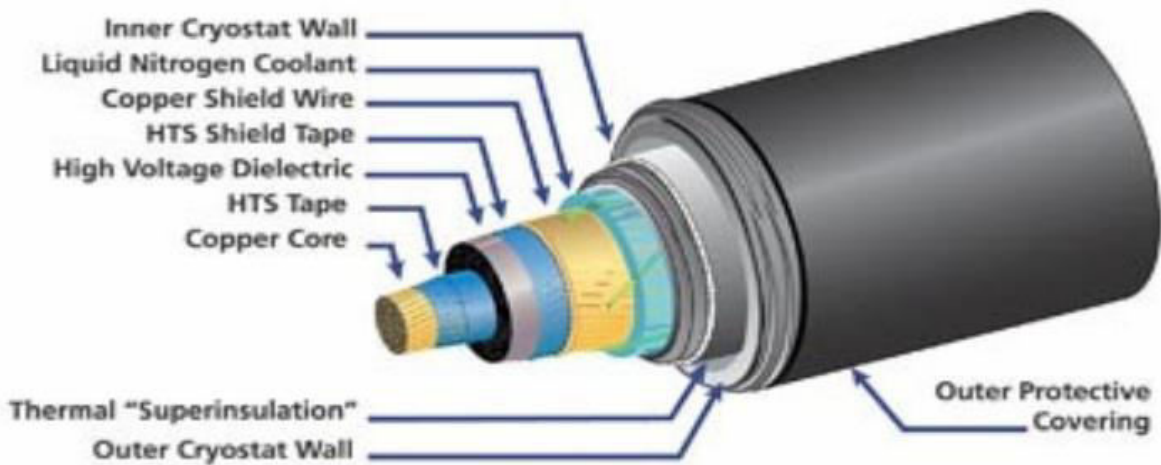
Figure 2-5 Schematic diagram of High Temperature superconducting (HTS) cable designed by NEXANS[8]
