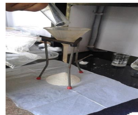
Fig.4.22 Angle of repose
