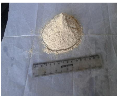
Fig.4.23 Measurement of radius
