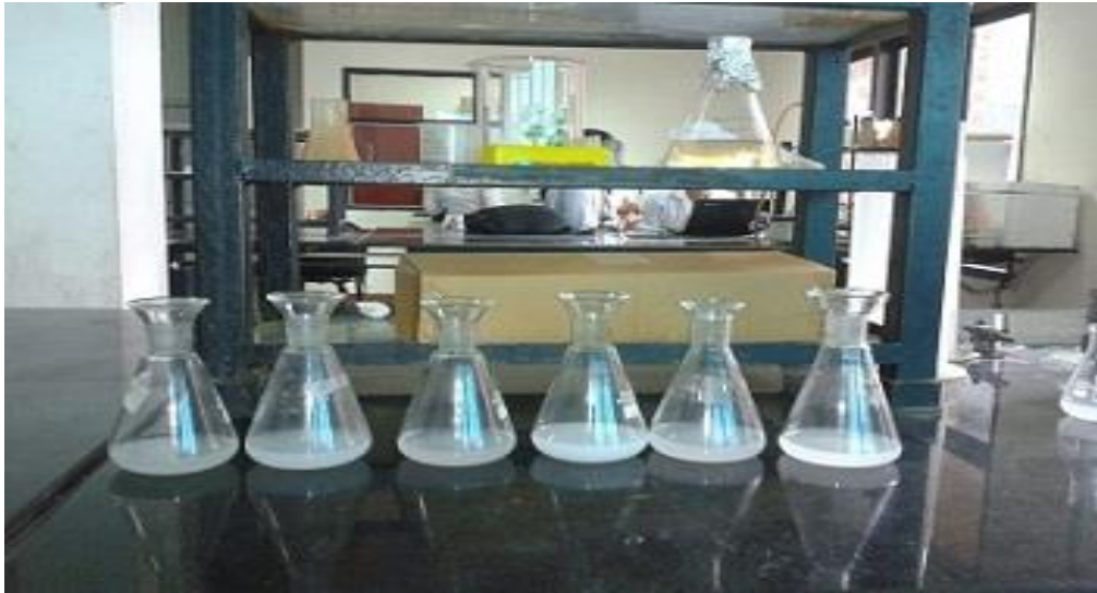
Fig 23: Result after titration of saponification value.
