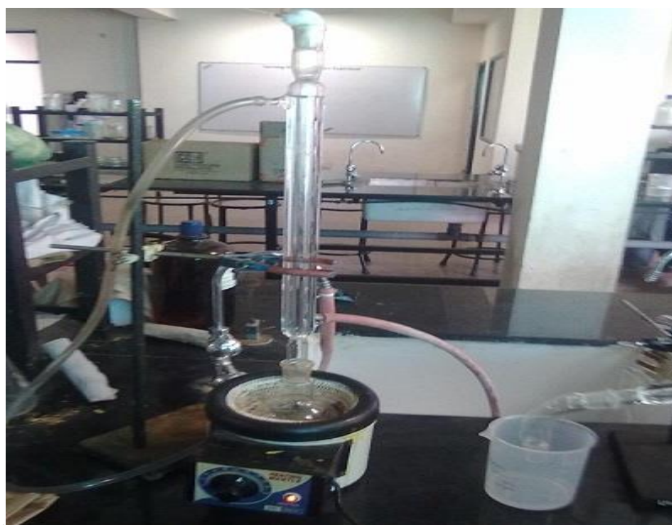
Fig 12: Transesterification Oil sample kept for Reflux.
