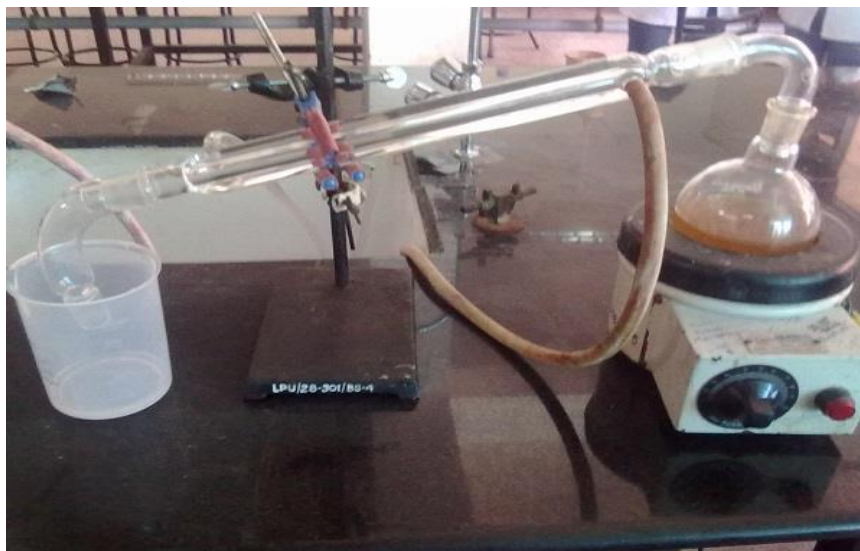
Fig 11: Distillation for separating oil and organic solvent ( n-hexane).
