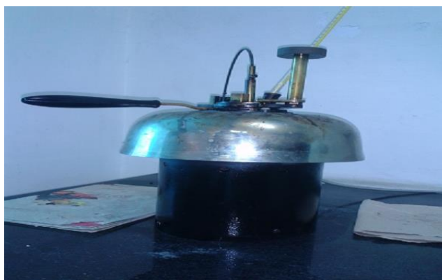
Fig 15: Pensky Martin apparatus used for the determination of fire and flash point.
