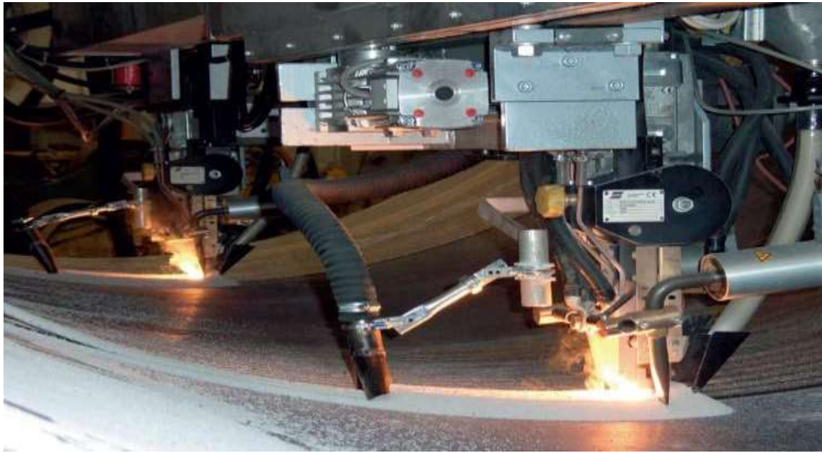
Figure 3.3 Cladding in Process on Low Carbon steel plate.[18]
