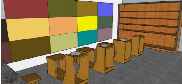
Fig. 48 working table with marble top for sheet Work and clay molding, trash box under the Table for used clay and P.O.P.
