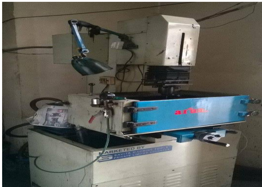
Figure 4.1 Experimental Setup of Die sinking EDM
