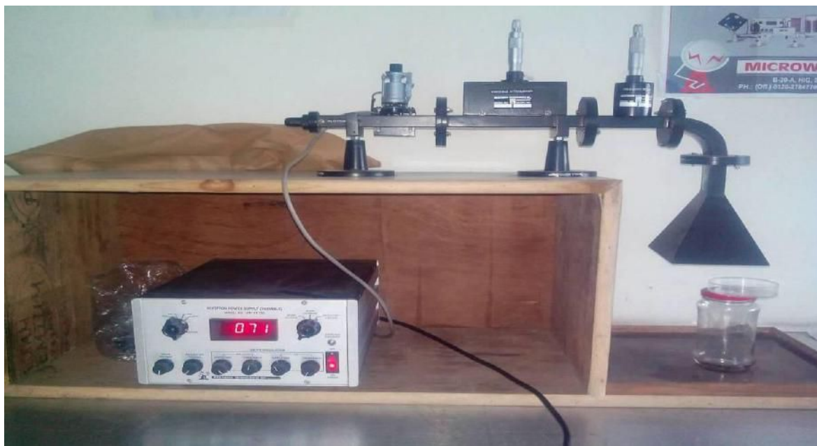
Figure no. 1 Klystron microwave test bench
