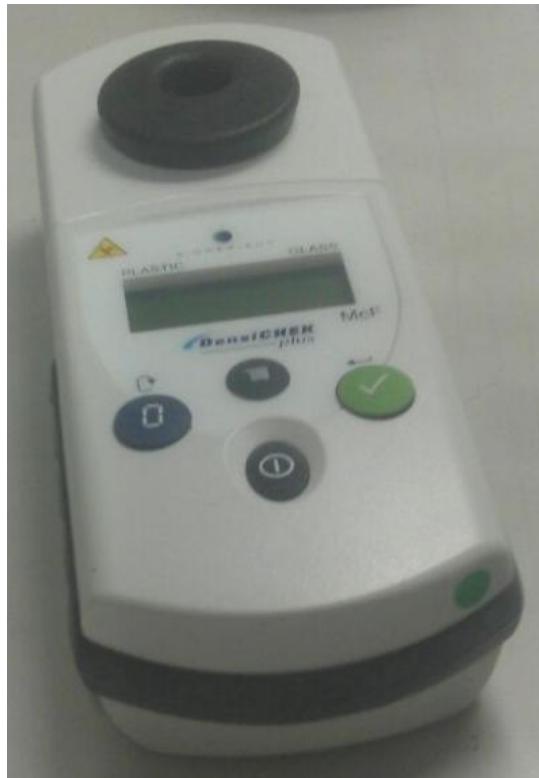
DensiChek used for measuring the turbidities.
