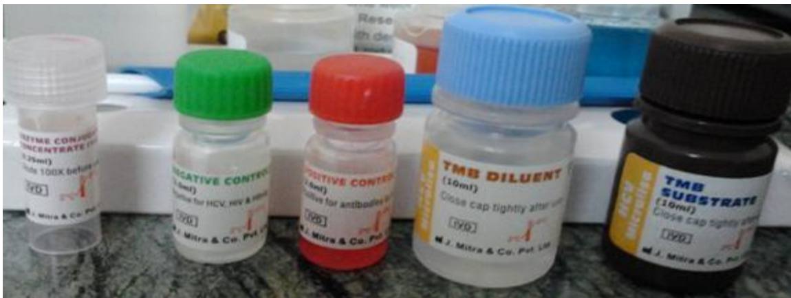
Figure 5: Components of the kit (Enzyme conjugate concentrate, negative control, positive control, TMB diluent and TMB substrate)
